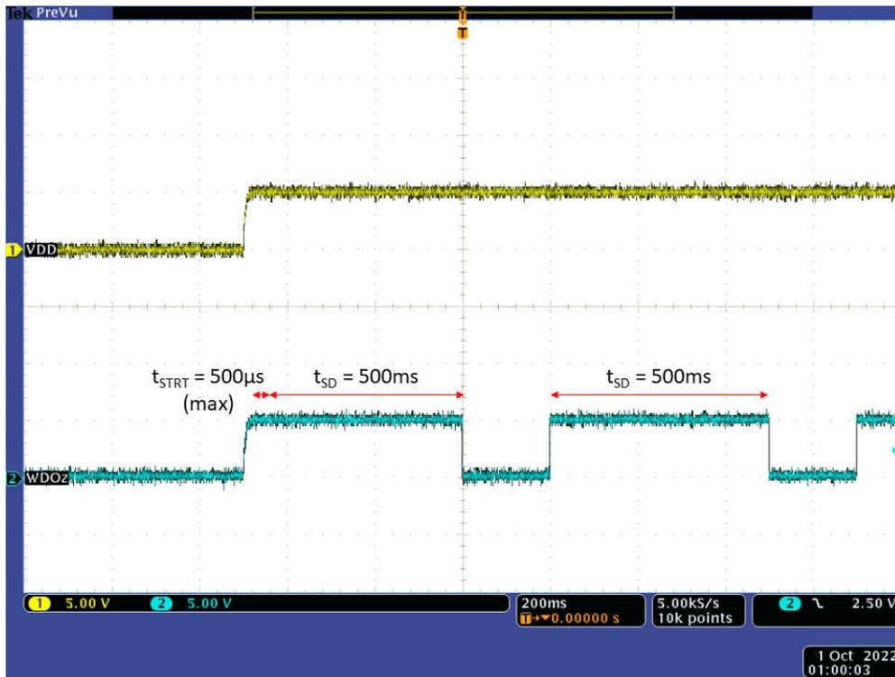
Figure 6-4. Startup Delay
