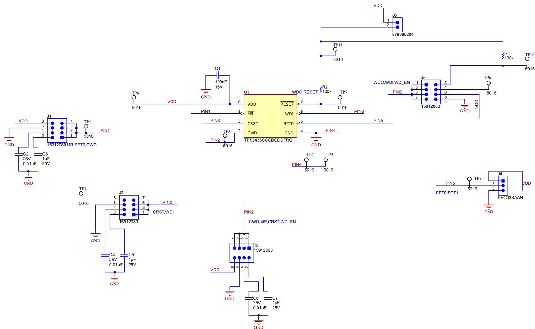
Figure 3-1. TPS36Q1EVM Schematic
