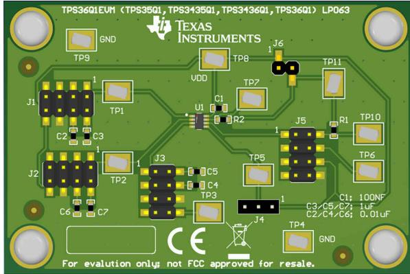
Figure 3-2. Component Placement—Top Assembly
