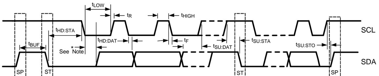
\* Note: SDA and SCL should be held low for 2  $\mu s$  after a Start condition to properly de-assert the Start indicator.
