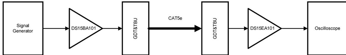
**Figure 9. Test Setup with the Cable Extender Chipset**
