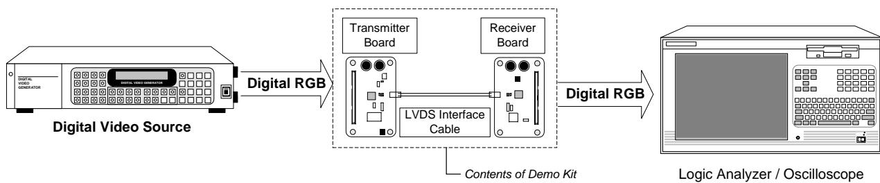
**Figure 5. Typical SERDES Test Setup for Evaluation**
