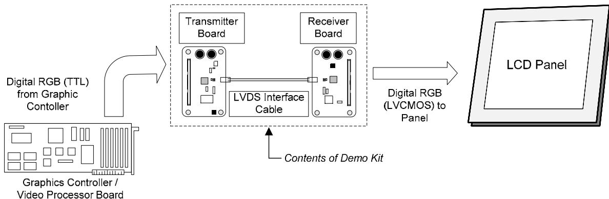
**Figure 4. Typical SERDES Setup of LCD Panel Application**
