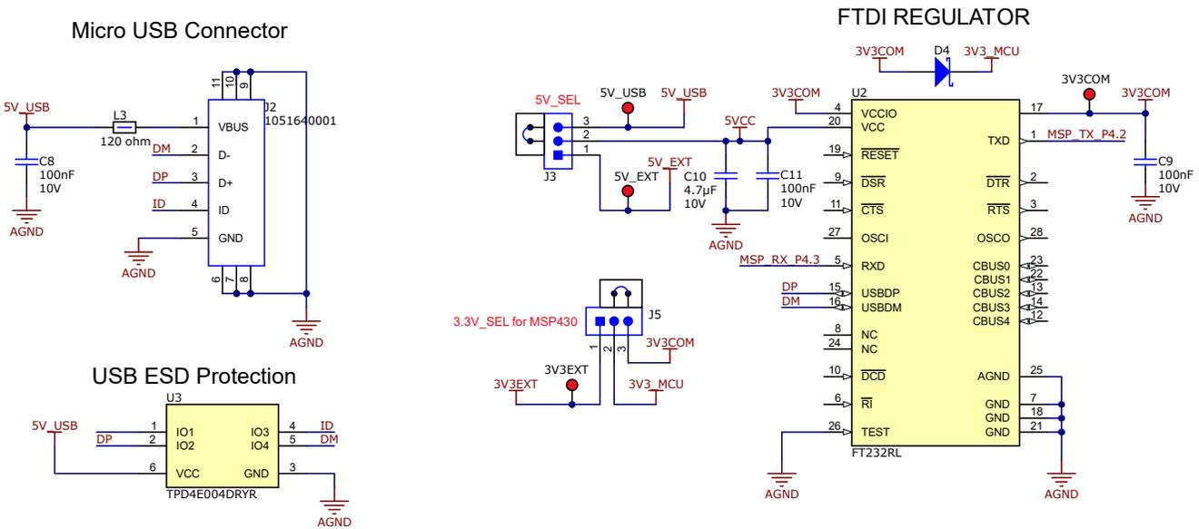
Figure 4-5. USB to UART Schematic
