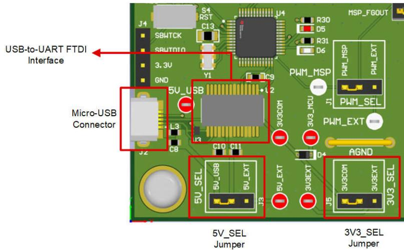
Figure 2-4. Micro-USB Connector and UART for MCT8315ZEV
