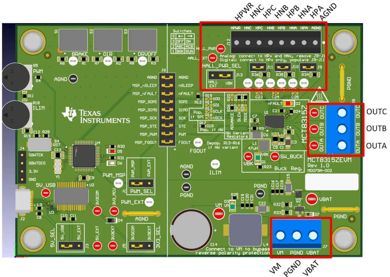
Figure 2-3. Connections from Motor to MCT8315ZEVM
