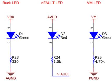
Figure 4-7. Status LEDs Schematic
