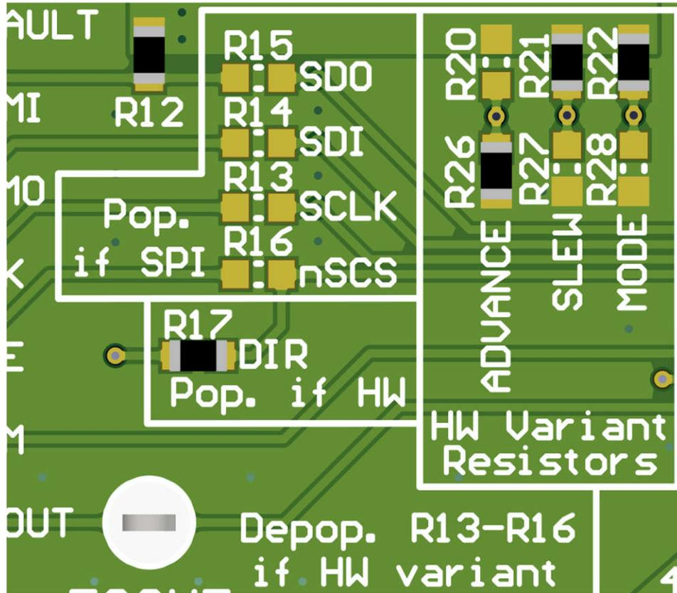
**Figure 2-7. Resistor Divider Settings for MCT8315ZH or MCT8315ZT (Hardware Variants)**
