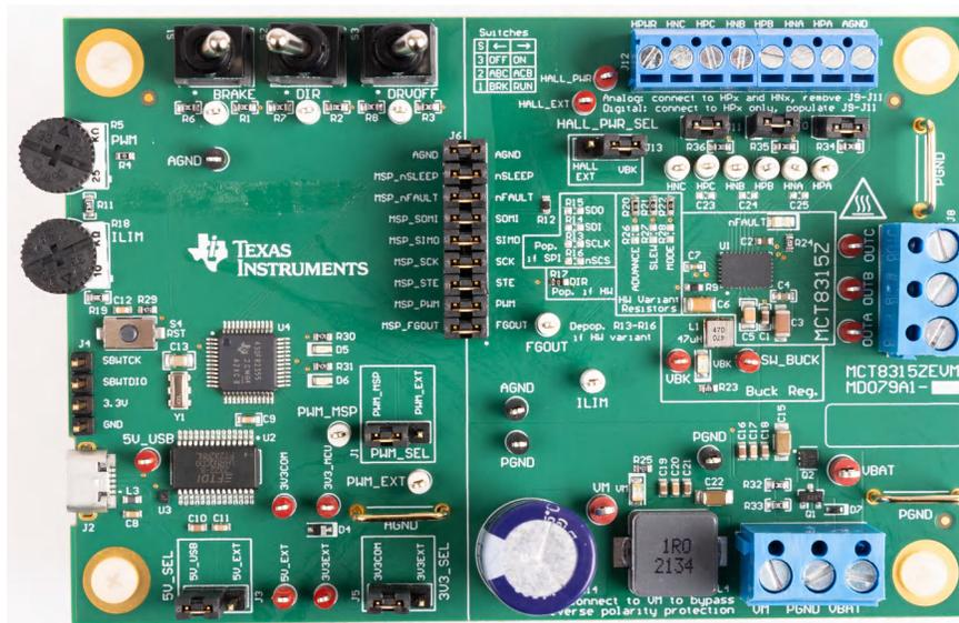
MCT8315ZEVM Printed Circuit Board (PCB - Top View)
