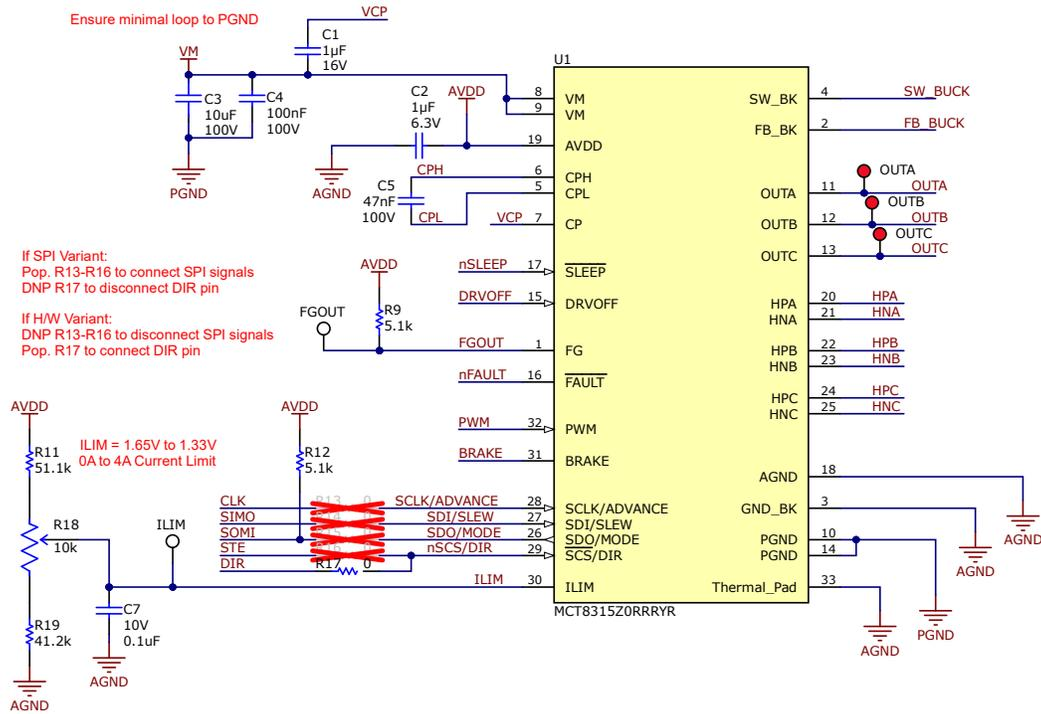
Figure 4-1. MCT8315Z 3-Phase Sensored Trapezoidal Motor Driver Schematic
