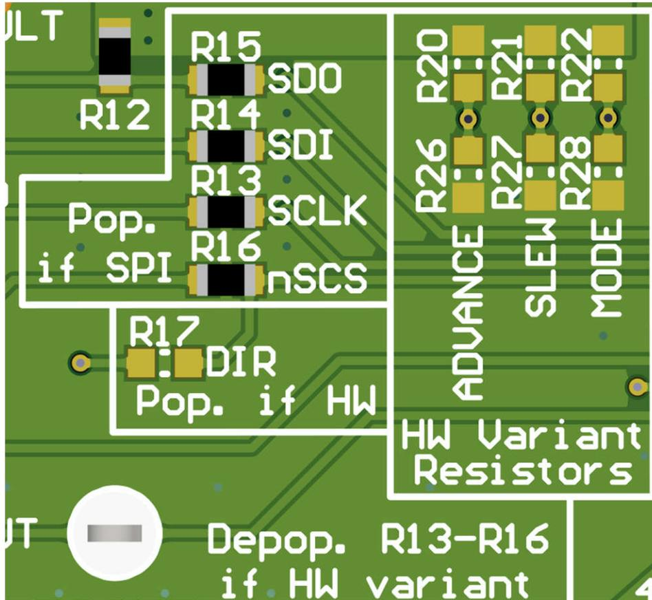
Figure 2-8. Resistors for MCT8315ZR (SPI variant)
