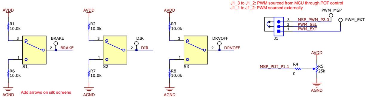
Figure 4-9. Switches and Speed Input Schematic
