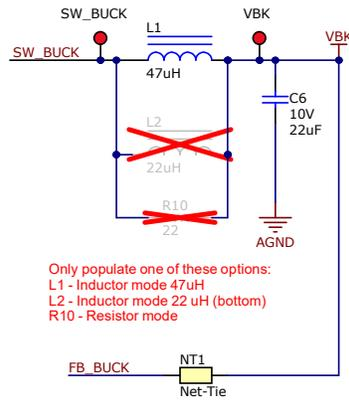
Figure 4-3. Buck Regulator Schematic
