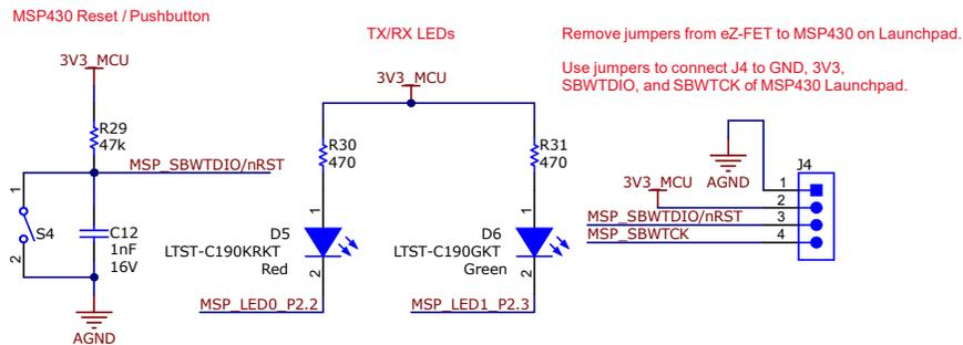
Figure 4-6. MCU Programming and Debug Schematic
