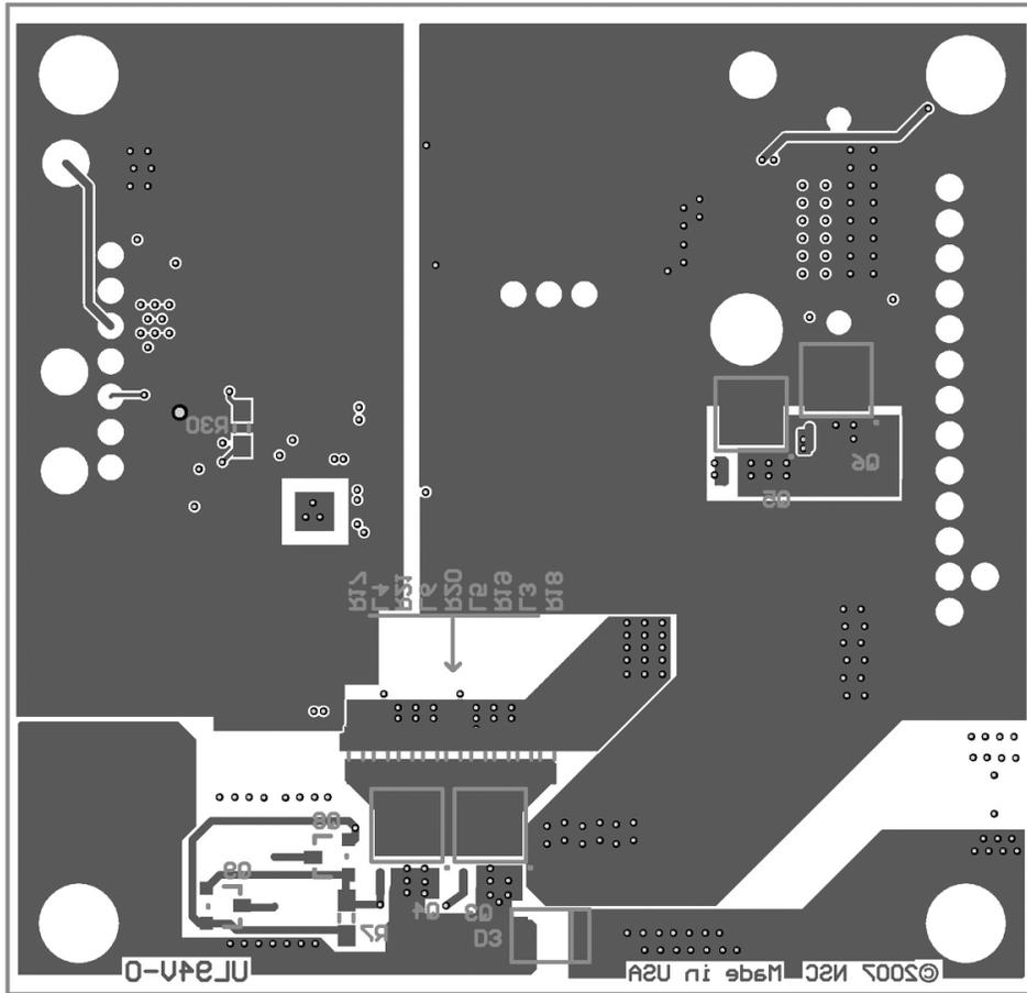
Figure 12. Bottom Layer and Bottom Overlay
