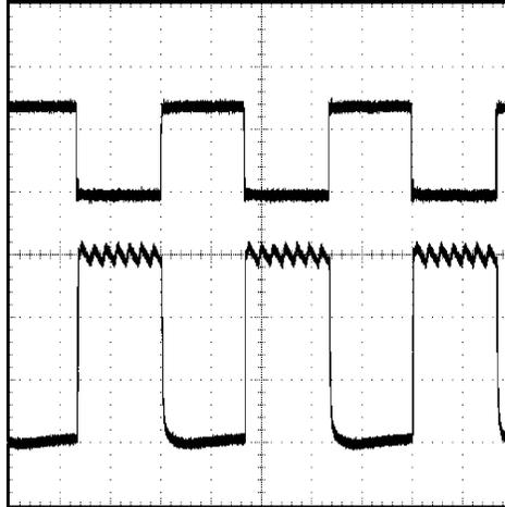
I<sub>LED</sub> = 6A nominal, V<sub>IN</sub> = 3.3V, V<sub>EE</sub> = -12V Top trace: DIM input, 2V/div, DC Bottom trace: I<sub>LED</sub>, 2A/div, DC T = 10 $\mu$ s/div
