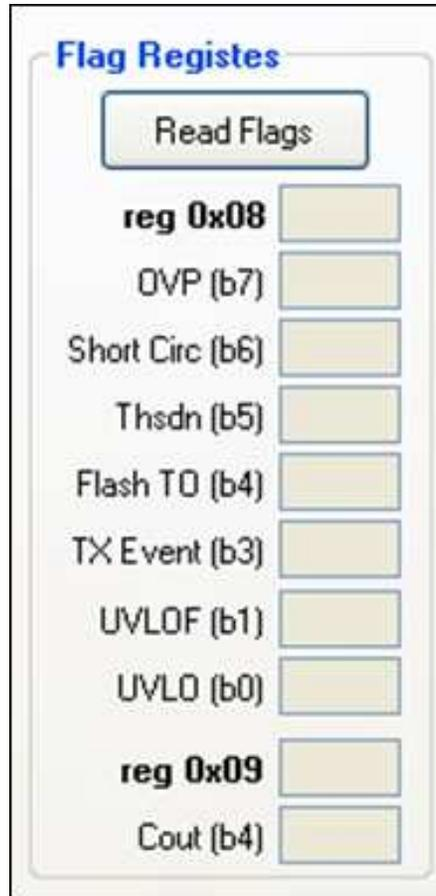
Figure 21. Fault Register
