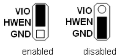
**Figure 1. Enable Jumper Settings**
