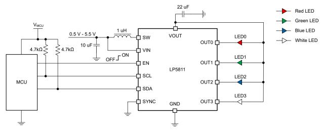
Figure 1-3. LP5811 Simplified Schematic
