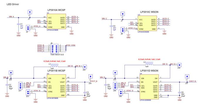
Figure 4-1. Schematic of LED Driver Module
