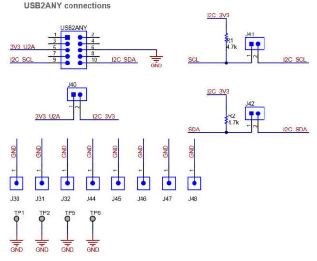
Figure 4-3. Schematic of USB2ANY and GND Connector
