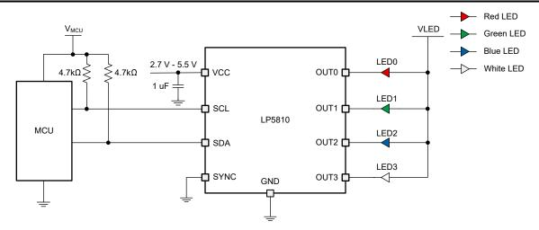
Figure 1-2. LP5810 Simplified Schematic
