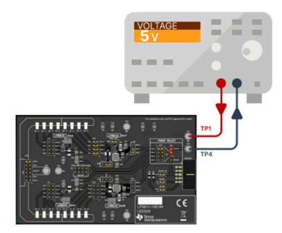
Figure 2-3. External Power Supply
