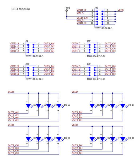
Figure 4-2. Schematic of LED Load Module
