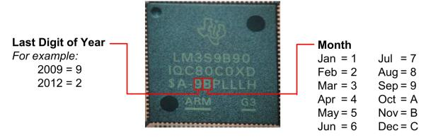
Figure 1. Example of Device Part Markings
