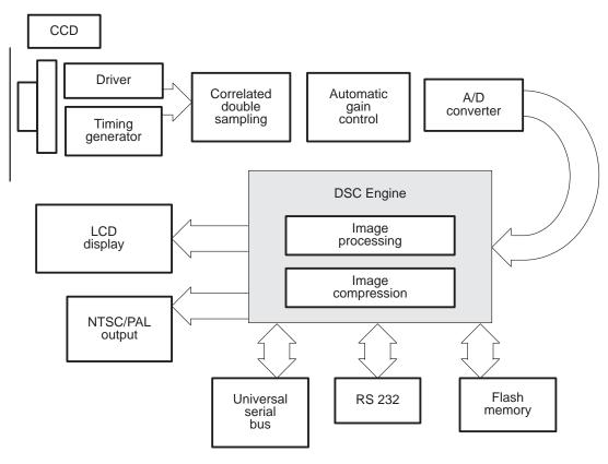
Figure 3. Digital Still Camera Block Diagram
