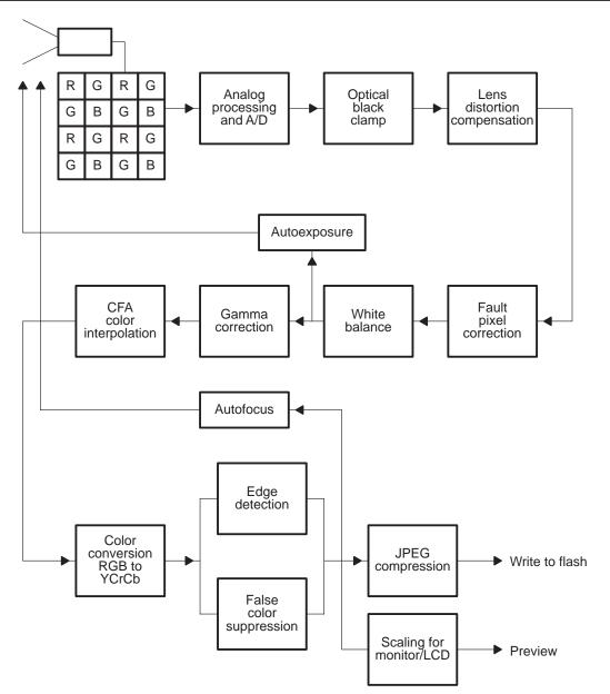
Figure 4. DSC Image Pipeline
