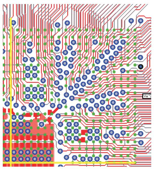
Figure 5. Second Quadrant Routing (top and bottom layers)
