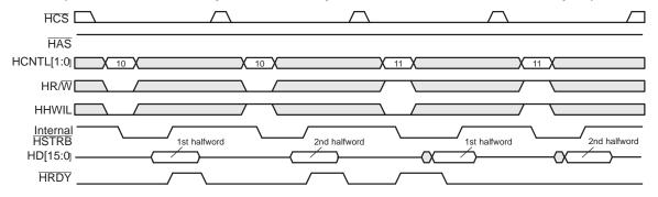
Figure 9 includes an autoincrement HPID read cycle. The host writes the memory address while asserting HCNTL[1:0] = 10b and reads the data while asserting HCNTL[1:0] = 01b. During the first HPID read cycle, HRDY goes high for only the first halfword access, and subsequent HPID read cycles do not cause HRDY to go high.
