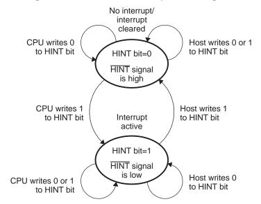
Figure 16. CPU-to-Host Interrupt State Diagram
