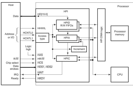
Figure 1. HPI Block Diagram
