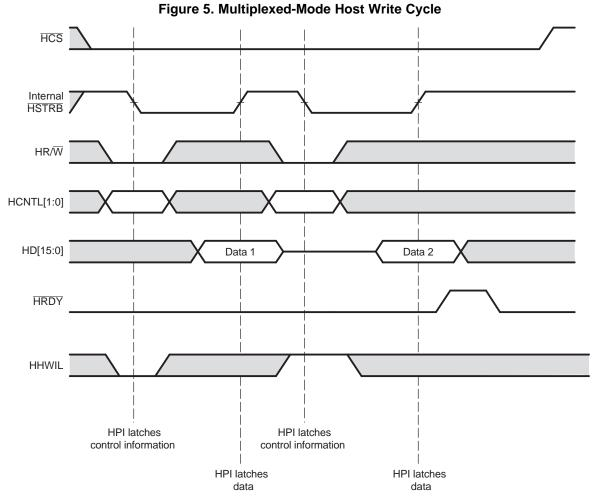
NOTE: Depending on the type of write operation (HPID without autoincrementing, HPIA, HPIC, or HPID with autoincrementing) and the state of the FIFO, transitions on HRDY may or may not occur. For more information, see Section 2.7.9.
