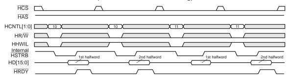
Figure 12 shows autoincrement HPID write cycles when the write FIFO is empty prior to the HPIA write. The host writes the memory address while HCNTL[1:0] = 10b and writes the data while HCNTL[1:0] = 01b. HRDY does not go high during any of the HPID write cycles until the FIFO is full.
