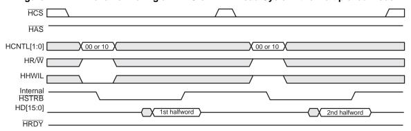
Figure 8 includes an HPID read cycle without autoincrementing. The host writes the memory address during the HPIA (HCNTL[1:0] = 10b) write cycle, and the host reads the data during the HPID (HCNTL[1:0] = 11b) read cycle. HRDY goes high for each HPIA halfword access, but HRDY goes high for only the first halfword access in each HPID read cycle.
