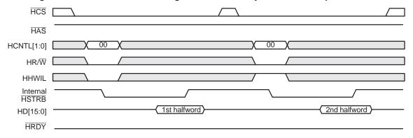
Figure 11 includes a HPID write cycle without autoincrementing. The host writes the memory address while HCNTL[1:0] = 10b and writes the data while HCNTL[1:0] = 11b. During the HPID write cycle, HRDY goes high only for the second halfword access.
