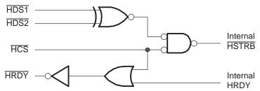
Strobe connections between the host and the HPI depend in part on the number and types of strobe pins available on the host. Table 2 describes some options for connecting to the HDS pins.
