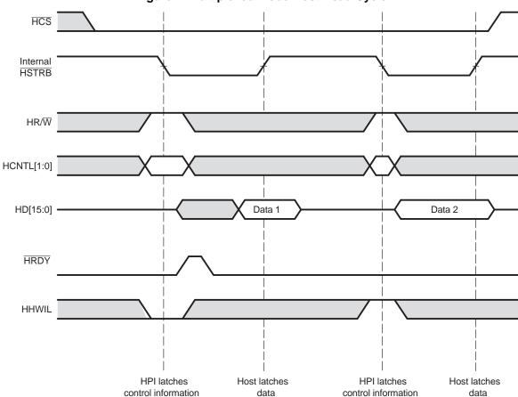
Figure 4. Multiplexed-Mode Host Read Cycle
