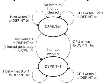
Figure 15. Host-to-CPU Interrupt State Diagram
