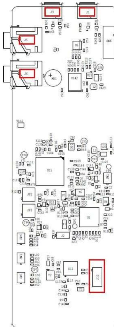
**Figure 28. Connectors on C5545 BoosterPack - Top**
