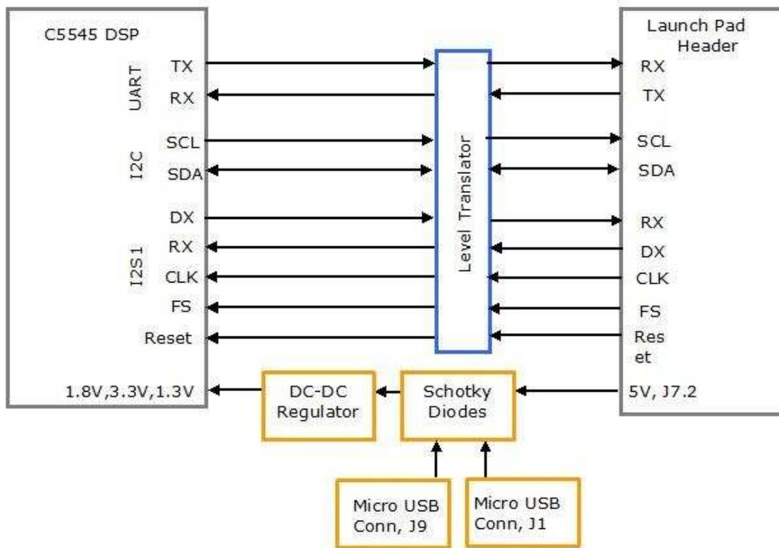
Figure 20. Connection Between C5545 and LaunchPad
