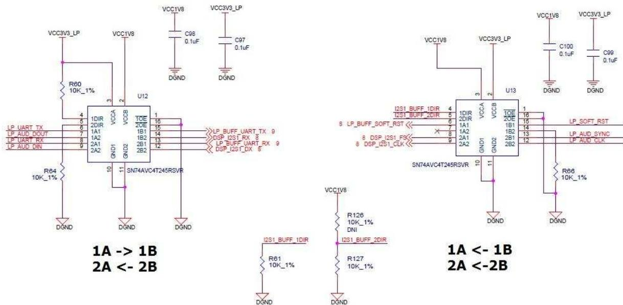
Figure 21. Level Shifter Direction for LP I2S and UART Interfaces
