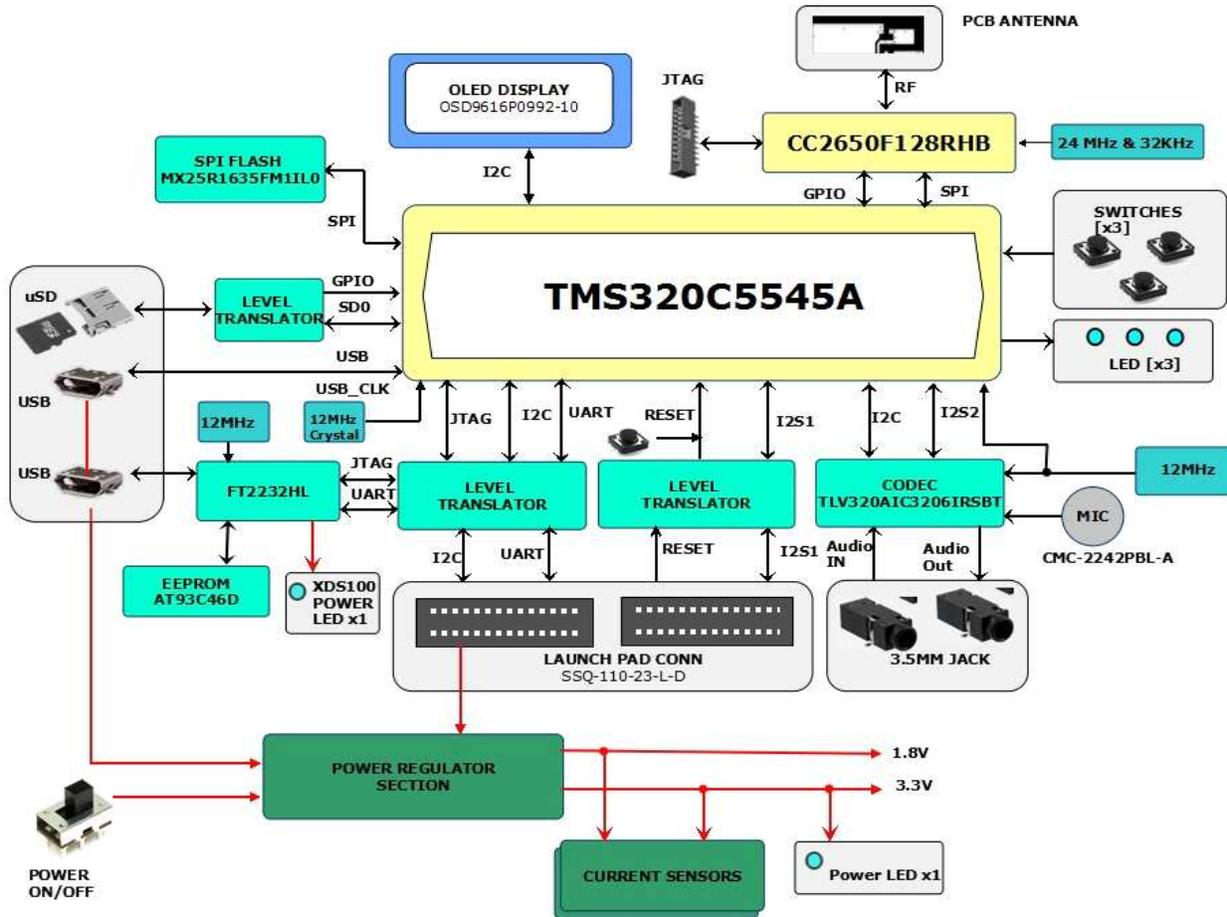
Figure 1. C5545 BoosterPack Functional Block Diagram
