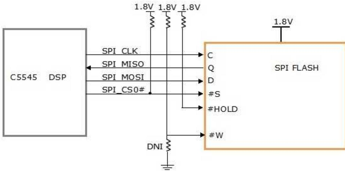
Figure 7. SPI FLASH Interface
