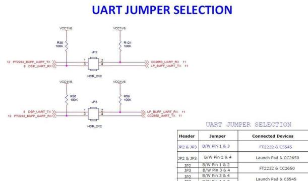
Figure 15. UART Interface - Schematics
