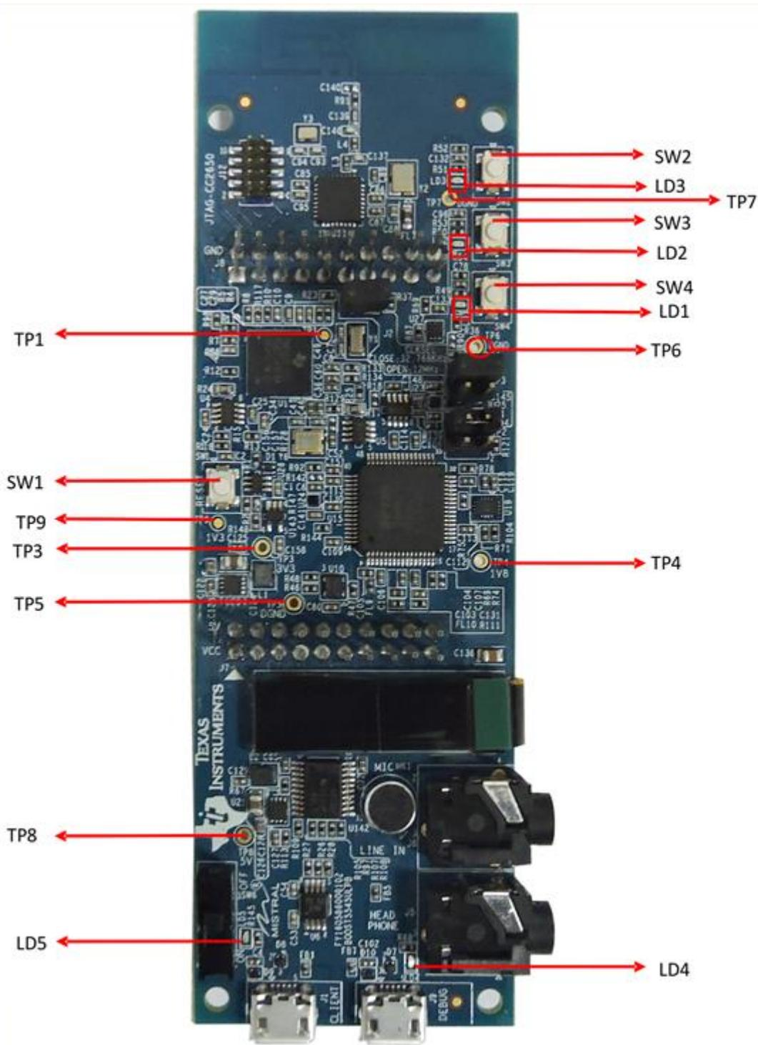
Figure 30. Position of LEDs, Test-Points and Push Buttons on the Board
