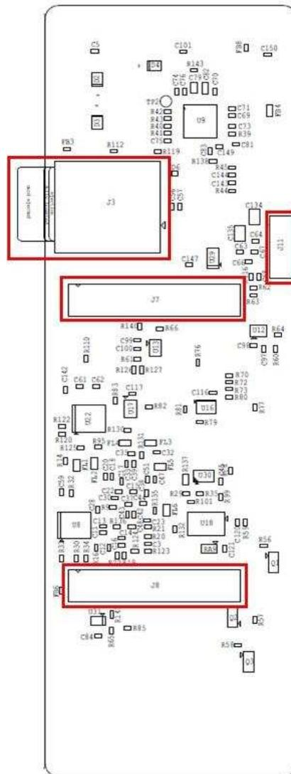
**Figure 29. Connectors on C5545 BoosterPack - Bottom**
