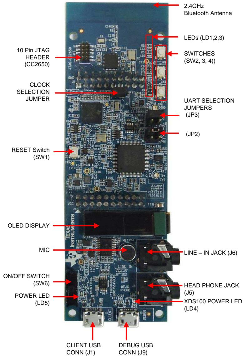
Figure 2. C5545 BoosterPack Top View
