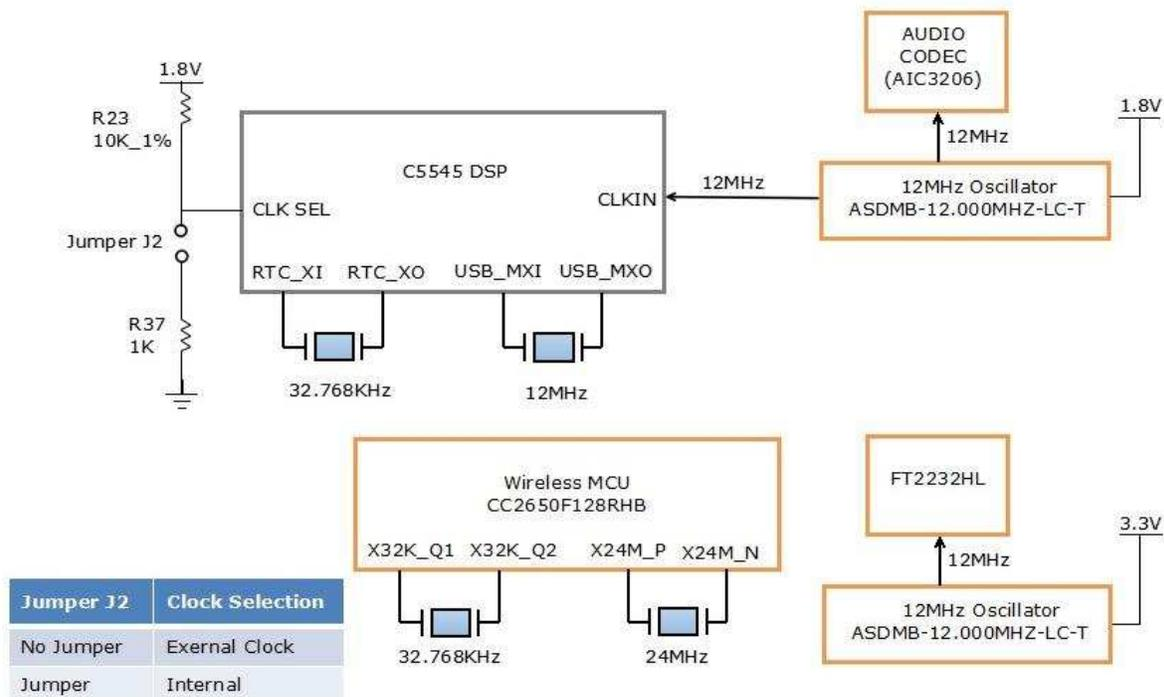
Figure 5. Clock Distribution and DSP Clock Selection
