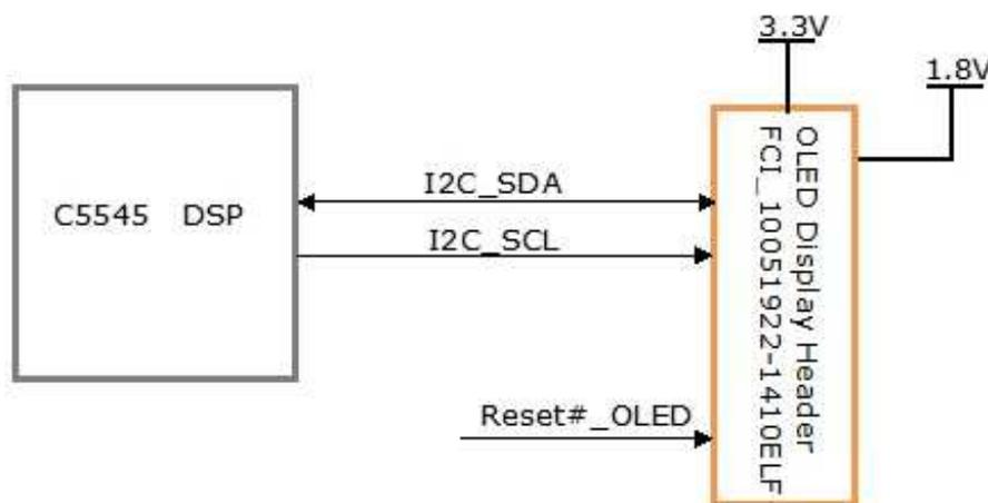
Figure 11. OLED Display Interface
