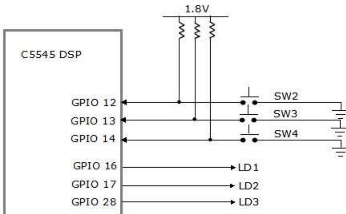
**Figure 8. Switch and LED Connection**
