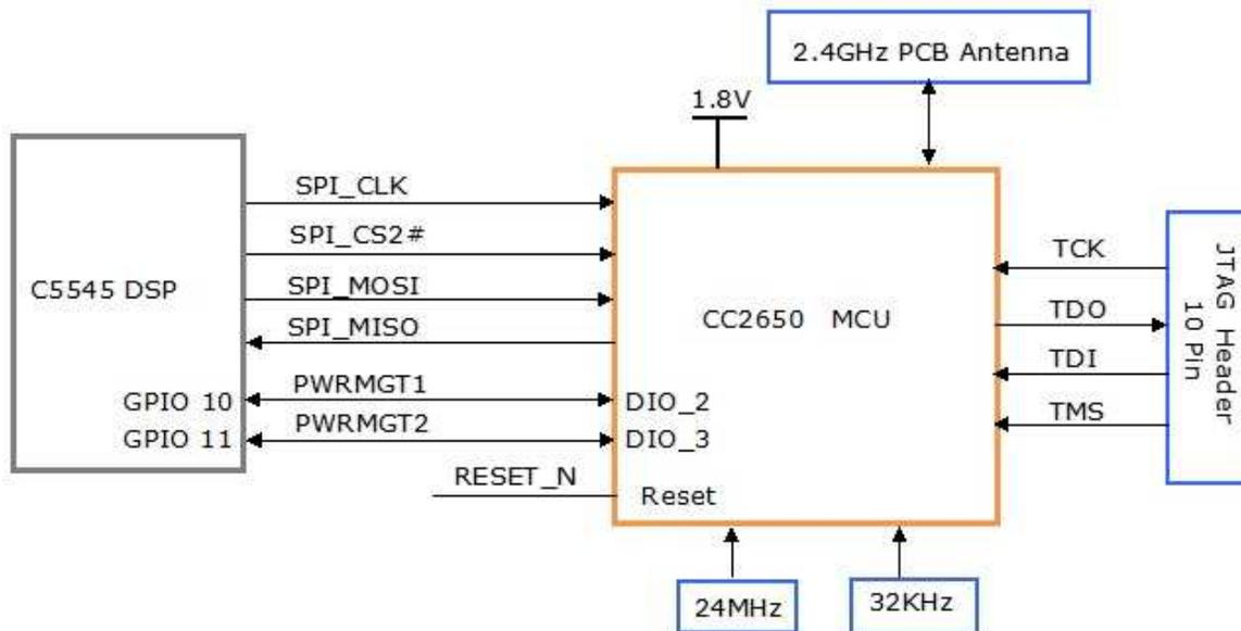
Figure 9. CC2650 SPI and GPIO Interface
