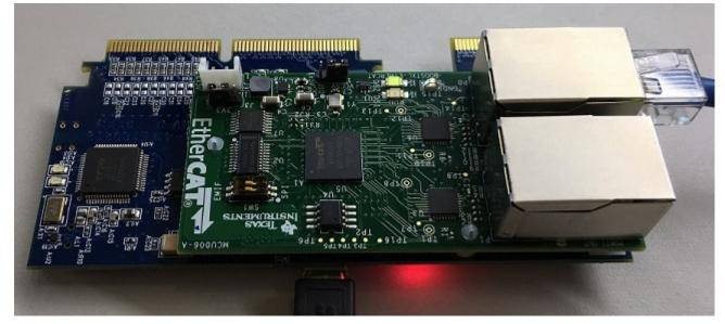
Figure 13. Stacked F28379D ControlCard + EtherCAT Adapter Board
