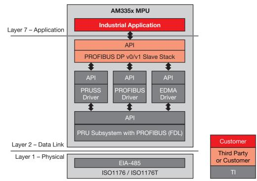
*Figure 6. Software architecture for PROFIBUS-DP*
