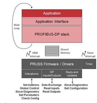
Figure 7. PROFIBUS® software integration
