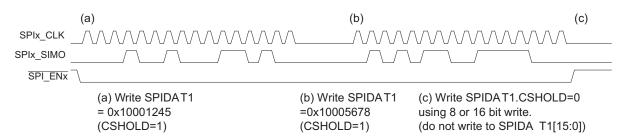
Figure 10. Workaround Assuming 32-Bit Writes to SPIDAT1 Followed by a Write Only to CSHOLD
