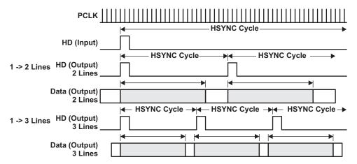
Figure 6. Readout Patterns Comparing Timing at the Output of the Reformatter
