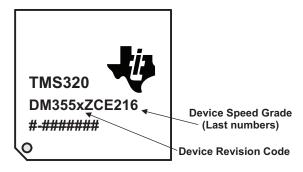
Figure 1. Example, Device Revision Codes for TMS320DM355 (ZCE)
