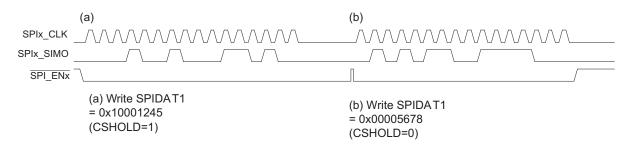
Figure 8. Actual CSHOLD Behavior-32-Bit Writes to SPIDAT1
