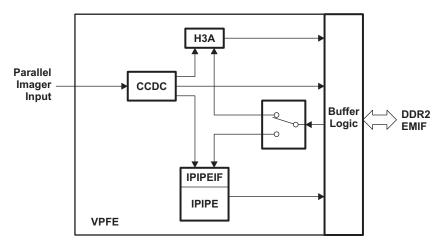
Figure 2. Video Processing Front End (VPFE) Block Diagram and Data Flows
