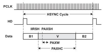
Figure 5. Paxel Width and Horizontal Paxel Count
