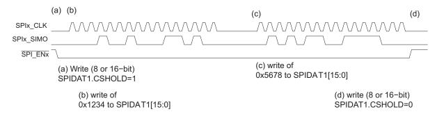
Figure 11. Workaround Assuming Halfword Writes to SPIDAT1
