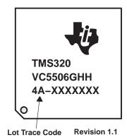
Figure 2. Example Markings for VC5506, GHH Package, Revisions 1.0 and 1.1
