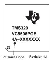
Figure 1. Example Markings for VC5506, PGE Package, Revisions 1.0 and 1.1
