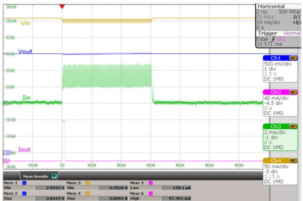
Figure 3. The pulse response of the TPS63900
