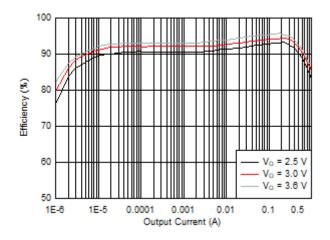
Figure 4. TPS63900 efficiency with an input voltage of 3.6 V
