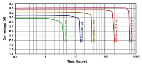
Figure 1. SAFT LS17330 typical discharge profiles at +20°C
