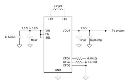
Figure 2. TPS63900 based battery front end
