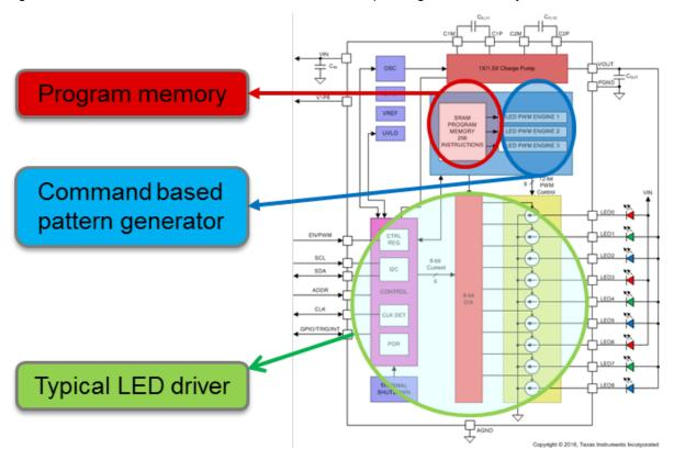
Figure 1. LED Driver Block Diagram
