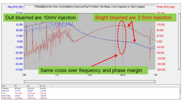
Figure 5. Bode Plot Comparison with Different AC Injection Magnitude
