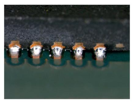
Figure 4. Toe Fillet on Standard QFN
