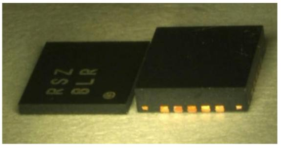
Figure 3. Standard QFN Package Side View
