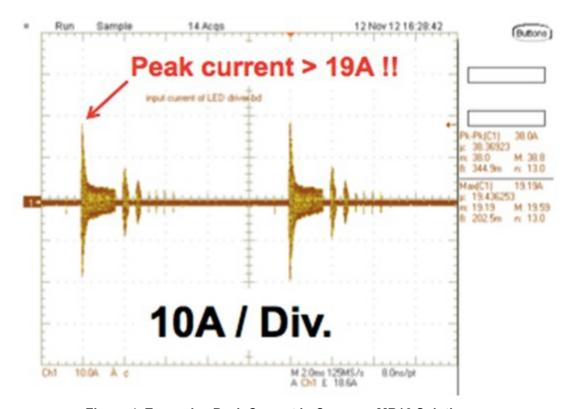
Figure 4. Excessive Peak Current in Common MR16 Solutions
