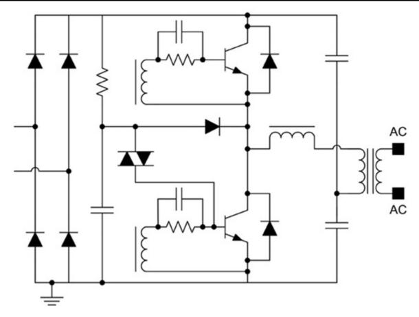
Figure 2. Electronic Low-voltage Transformer (ELVT) Circuit Diagram
