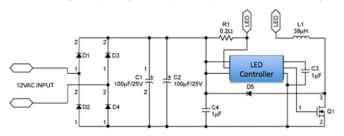
Figure 3. Typical MR16 Schematic
