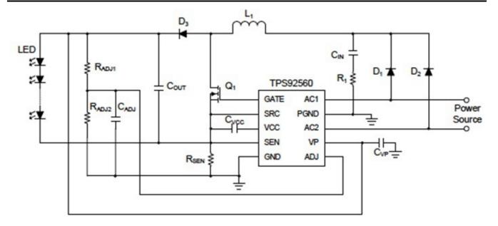
Figure 5. Input Capacitor Free MR16 Lighting with TPS92560
