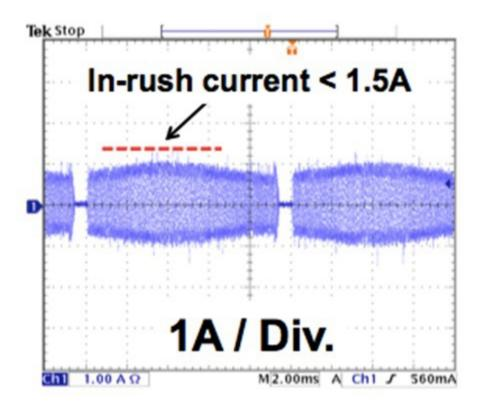
Figure 6. Peak Inrush Current with TPS92560
