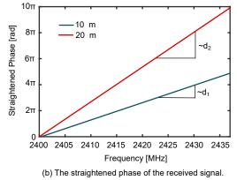
Figure 8-2. Measured Phase vs. Tone Frequencies (Wrapping Around 2π)
