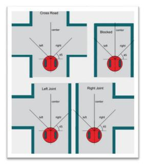
Figure 1. Eight possible scenarios as the robot explores the maze. As the robot approaches an intersection, it first determines what alternative paths exist, and then it chooses which way to go
