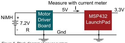
Figure 6. Block diagram of power system.
