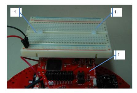
Figure 5. Solderless breadboard attached to the robot.
