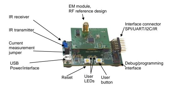
Figure 4-3 Target module layout
