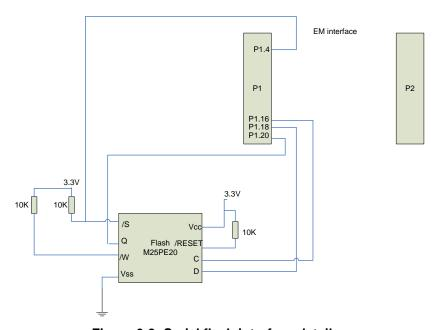
Figure 6-2: Serial flash interface details
