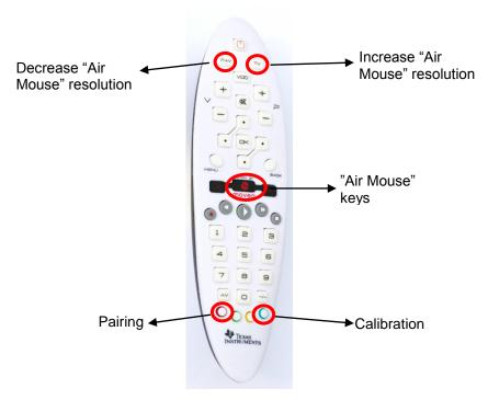
Figure 4-1: Remote Control Key layout
