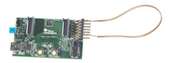
Figure 8-1: Short pin 1(GND) and pin11 (SDA)
