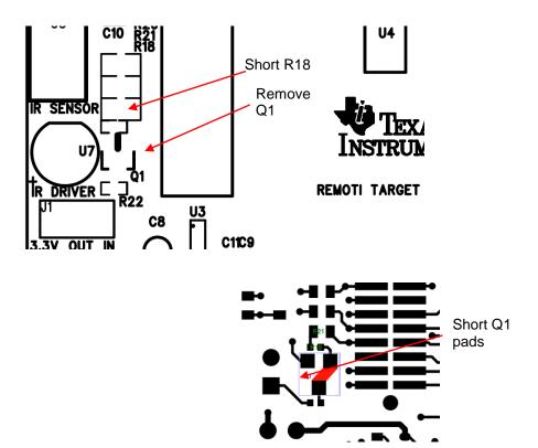
Figure 6-3: Changing polarity of IR control signal to active high
