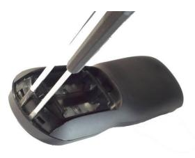
Figure 7-3: Opening the remote control, step one
