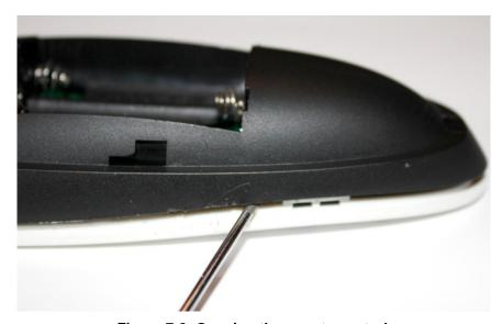
Figure 7-2: Opening the remote control
