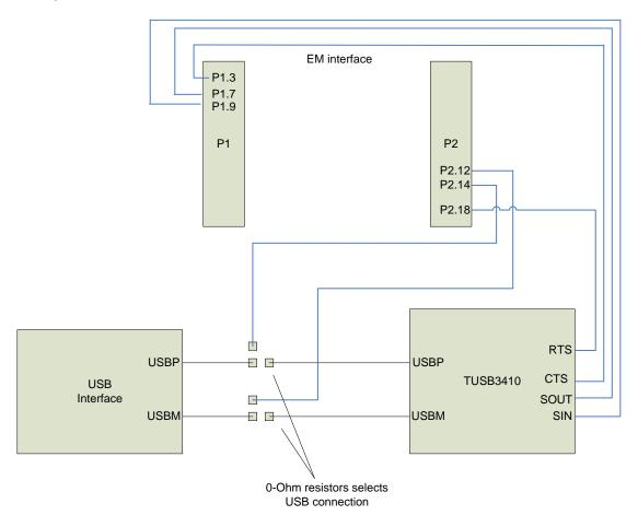
Figure 6-1: USB interface selection with 0-ohm resistor
