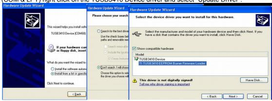
Figure 8-2: Installing the EEPROM burner driver
