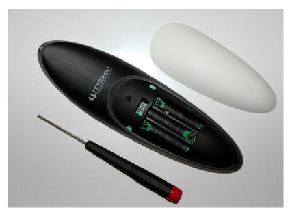
Figure 7-1: Tools for opening the remote
