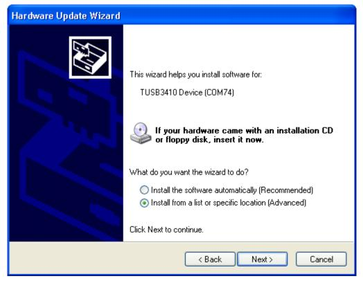
Figure 4-6: Select automatic installation of software (Windows XP)
