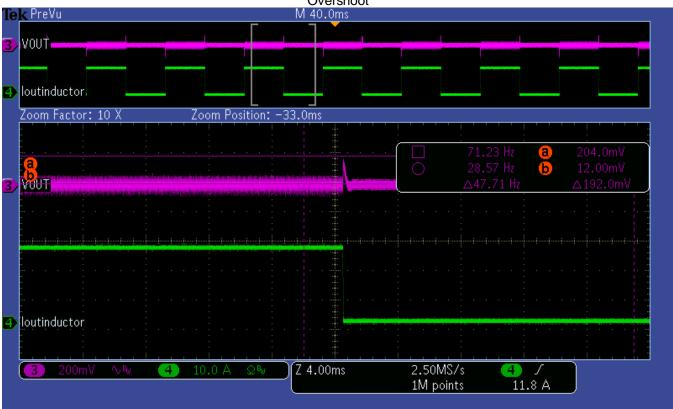
60.0Vin 12V Load from 0A to 25A to 0A, 20Hz, 2.5A/us.
