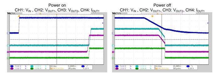
The waveforms of system power on and off with full load outputs are shown in following pictures.
