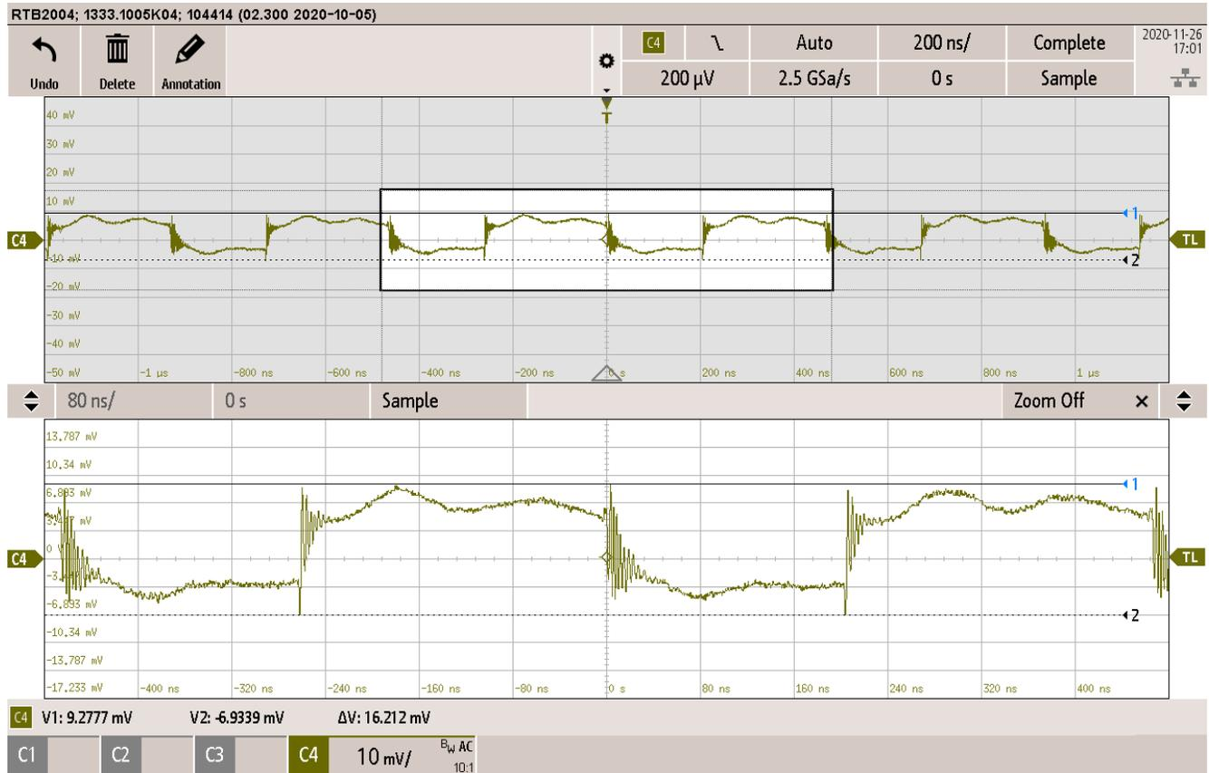
Figure 4-3. LMR50410-Q1 Output Voltage Ripple in CCM Mode
