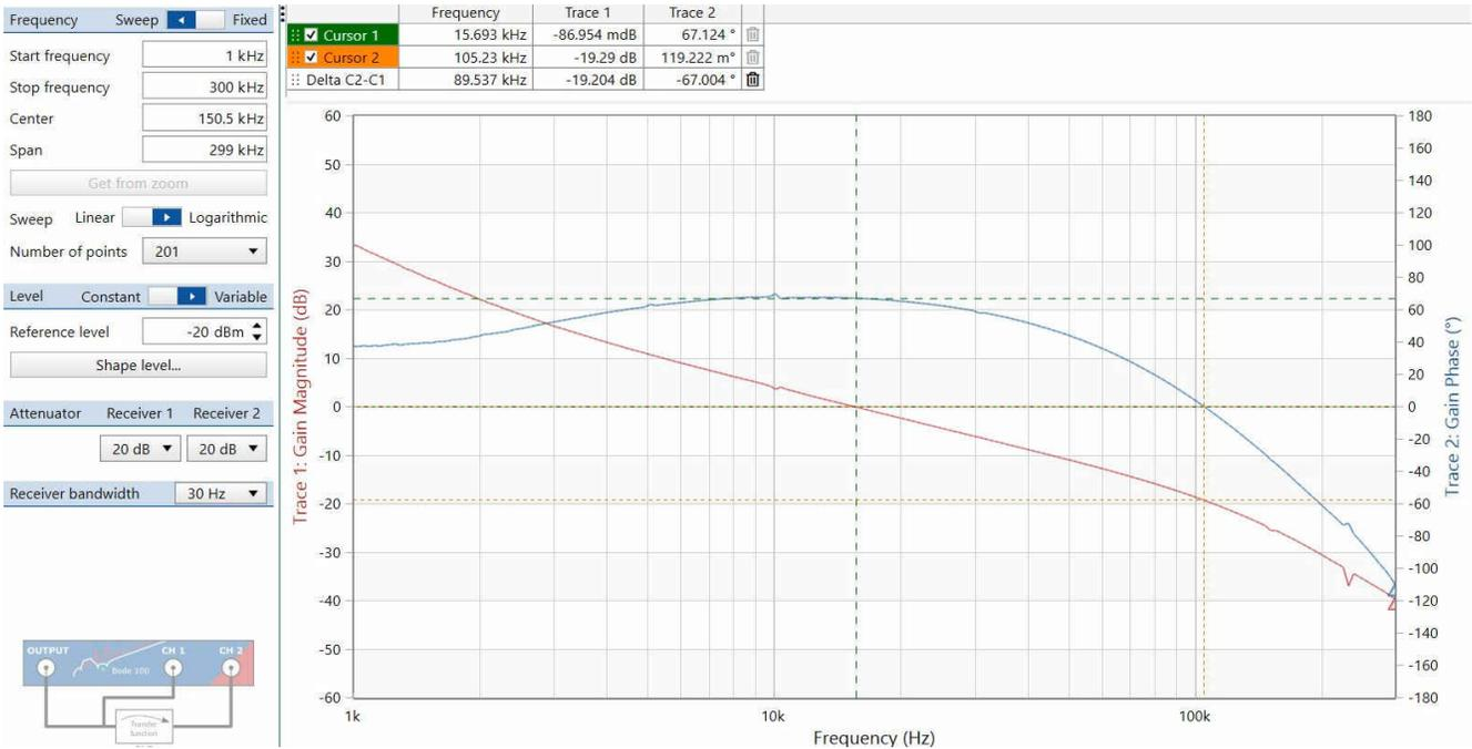
Crossover at 16 kHz with 67 degrees of phase margin, -180 degrees shift at 105 kHz with 19-dB gain margin
