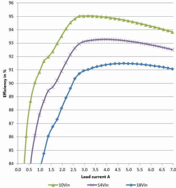
Figure 2-1. PMP23194 3.3-V DC/DC Converter Efficiency
