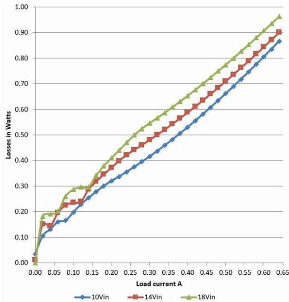
**Figure 2-6. PMP23194 8-V DC/DC Converter Losses**
