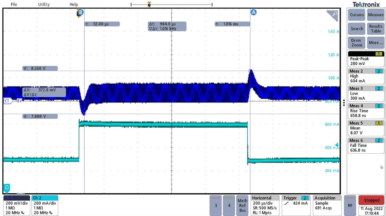
Undershoot and overshoot are each about 120 mV (dark blue trace). Dynamic current was measured with clip-on current probe (blue trace).
