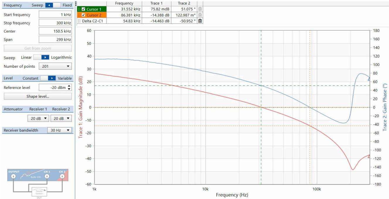
Crossover at 32 kHz with 51 degrees of phase margin, -180 degrees shift at 86 kHz with 14-dB gain margin
