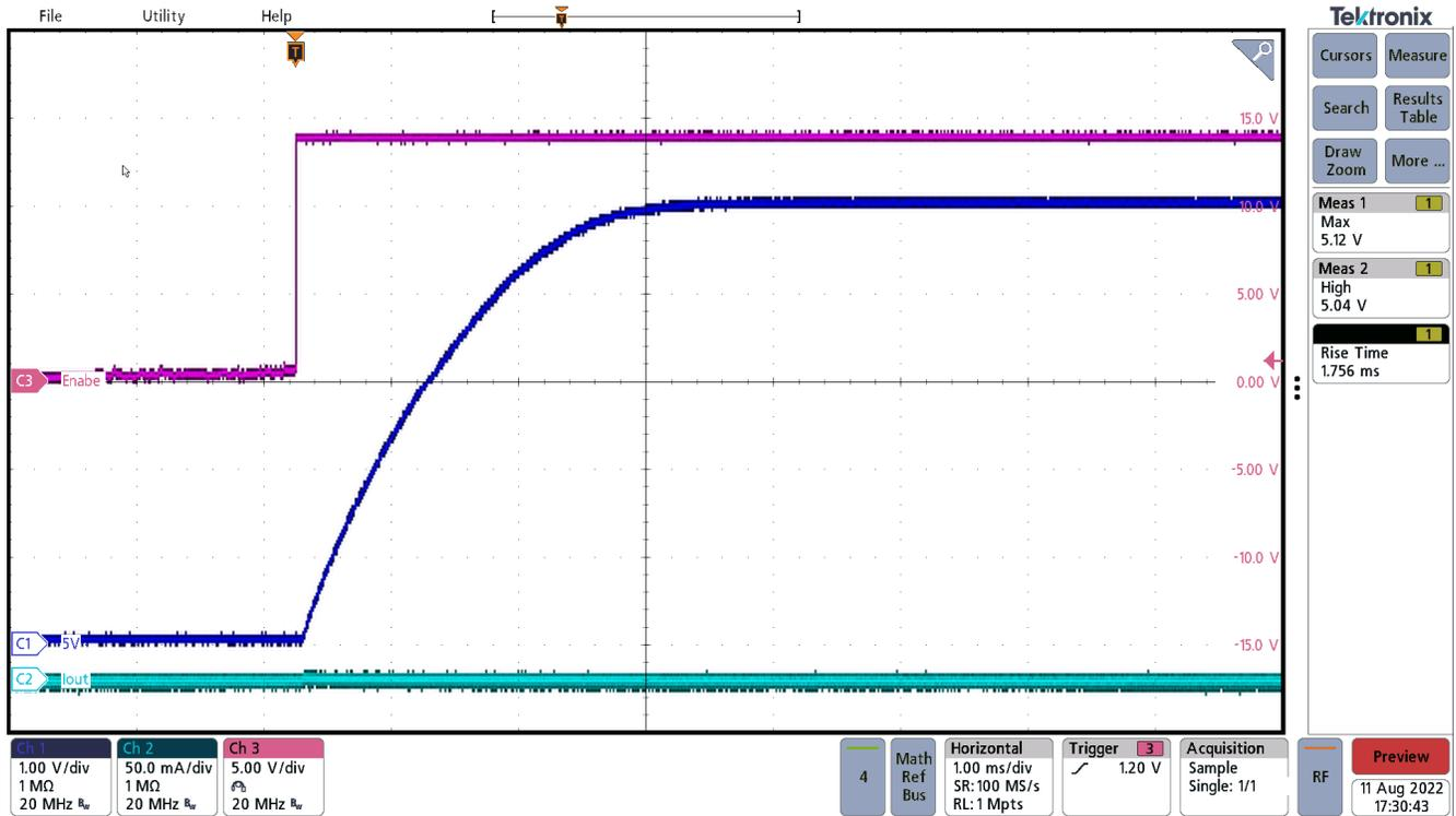
Enable going high: Enable going high: the red trace is the enable signal, the dark blue trace is  $V_{OUT}$ , and the light blue trace is the load current. Smooth 5  $V_{OUT}$  rise in under 3 ms with no overshoot seen.
