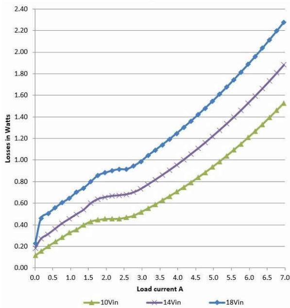
**Figure 2-4. PMP23194 3.3-V DC/DC Converter Losses**
