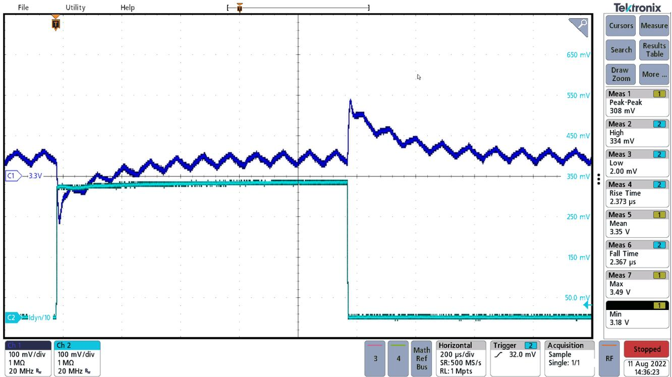
Output undershoot and overshoot each about 150 mV (purple trace). Dynamic current measured at J300 across a 100-mΩ shunt R306 on the PMP23194 board (blue trace).
