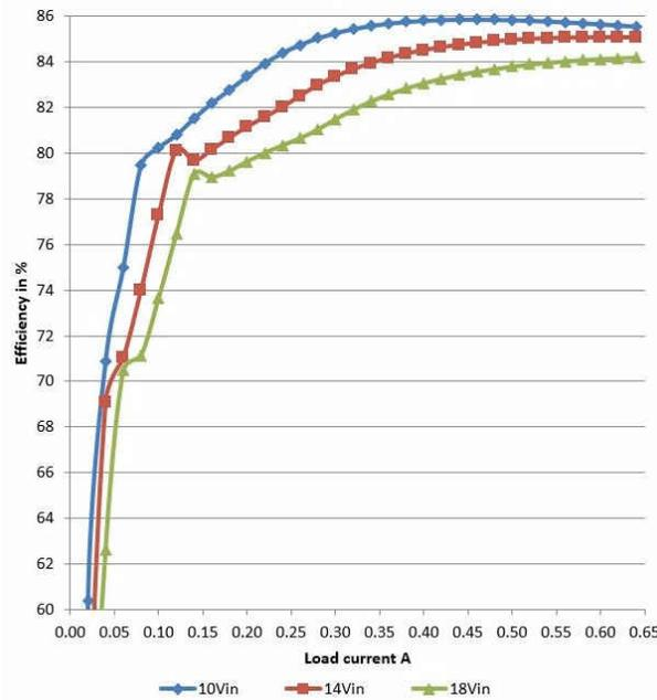
Figure 2-3. PMP23194 8-V DC/DC Converter Efficiency
