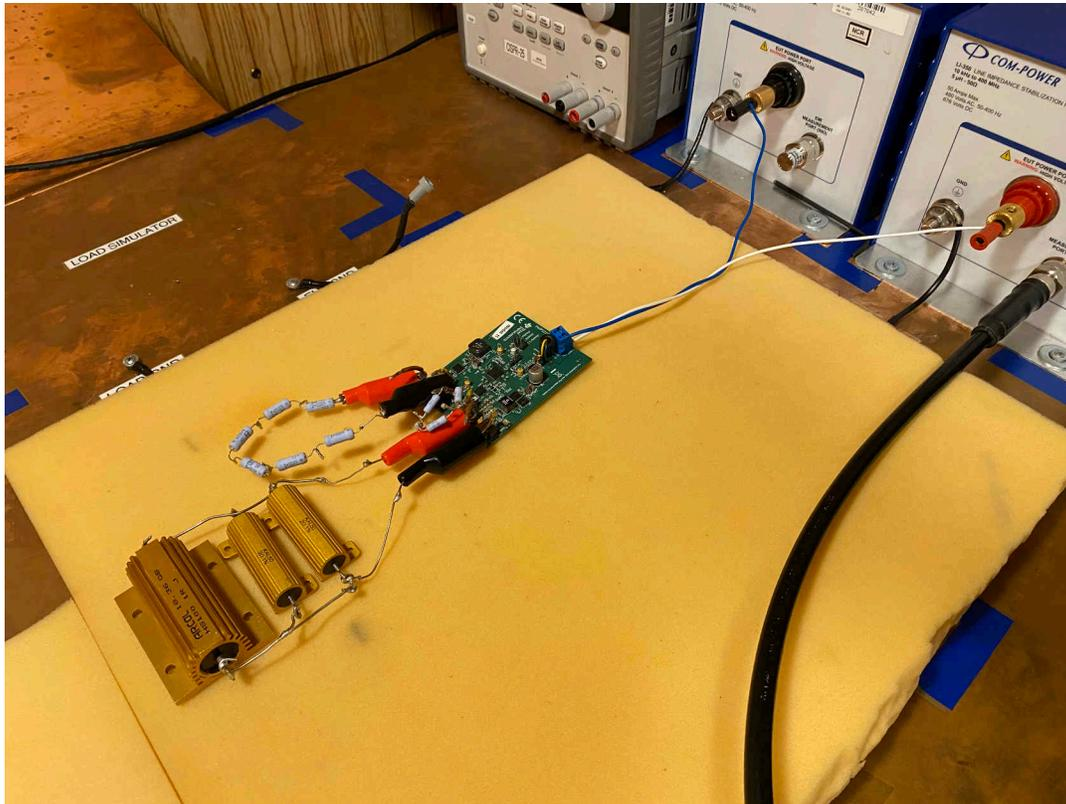
**Figure 1-1. Test Setup for Conducted Emissions**
