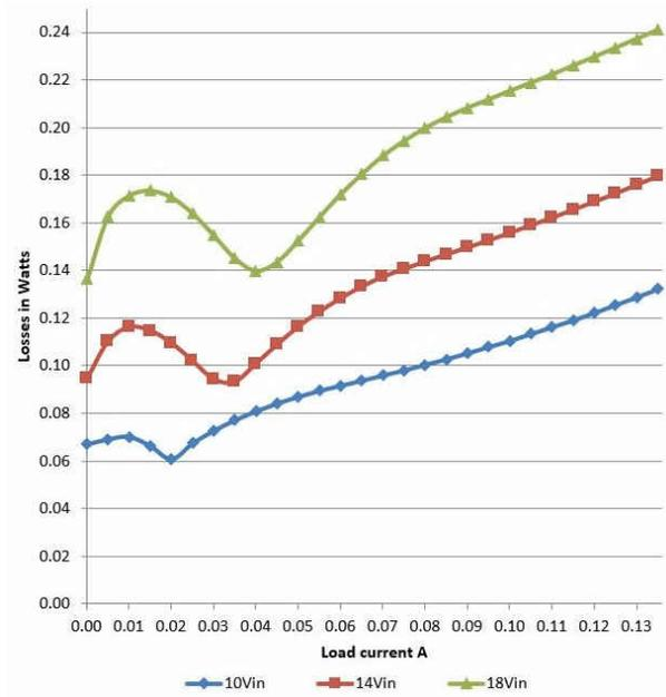
**Figure 2-5. PMP23194 5-V DC/DC Converter Losses**
