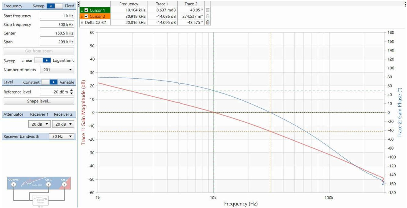
Crossover at 10 kHz with 49 degrees of phase margin, -180 degrees shift at 31 kHz with 14-dB gain margin
