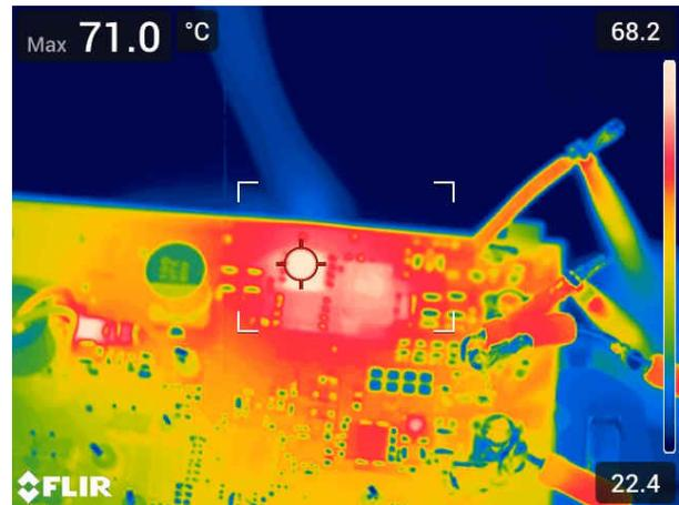
**Figure 2-8. High-Side FET Q4 of the 3.3-V Buck Converter Worst Case at 18 V<sub>IN</sub>, 71°C**
