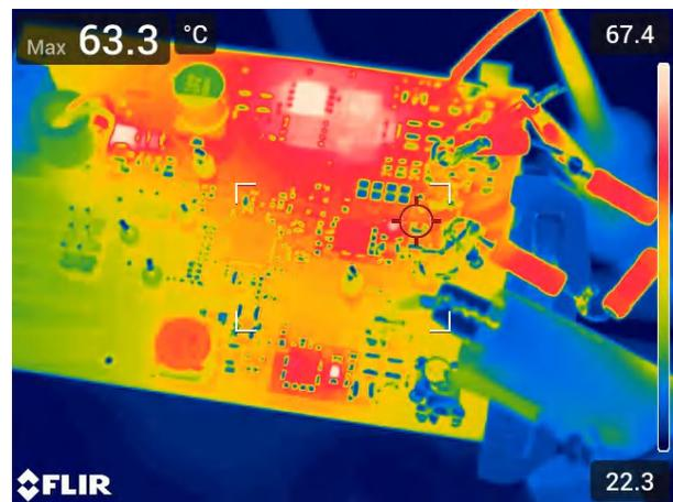
**Figure 2-10. Main Inductor of the 5-V Buck L2 Worst Case at 18 V<sub>IN</sub>, 63°C**
