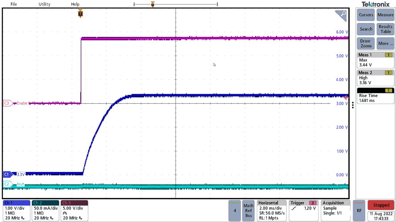
Enable going high: Red trace is the enable signal, the dark blue trace is  $V_{OUT}$ , and the light blue trace is the load current. Smooth  $V_{OUT}$  rise in under 2.5 ms with no overshoot seen.
