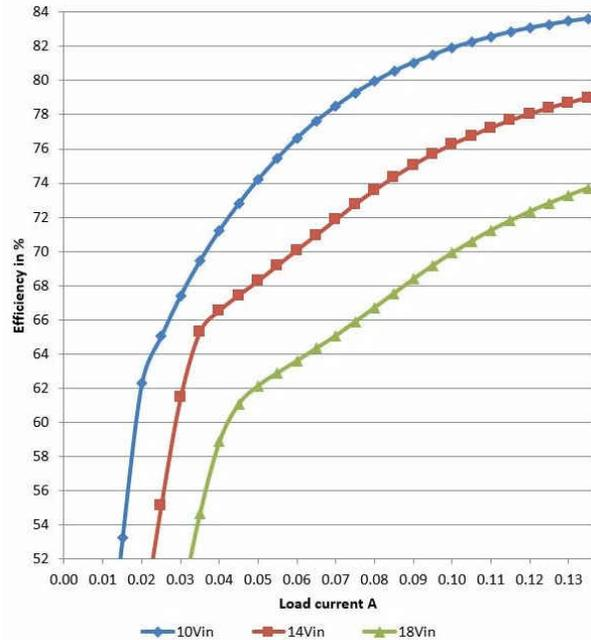
Figure 2-2. PMP23194 5-V DC/DC Converter Efficiency
