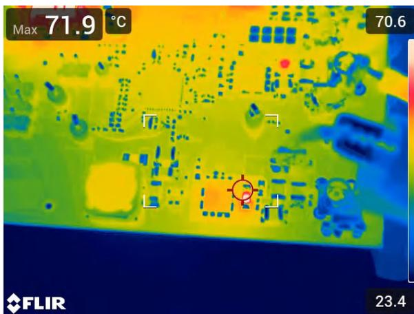
**Figure 2-9. Output Rectifier of the 8-V SEPIC D2 Worst Case at 10 V<sub>IN</sub>, 72°C**
