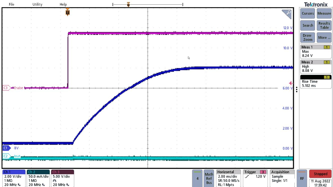
Enable going high: Enable going high: the red trace is the enable signal, the dark blue trace is  $V_{OUT}$ , and the light blue trace is the load current. Smooth 8  $V_{OUT}$  rise in under 10 ms with no overshoot seen.
