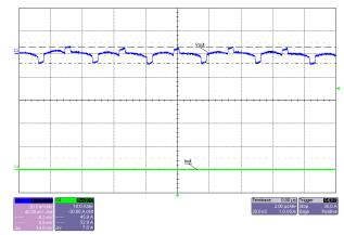
Figure 3-13. Output Voltage Ripple, 48V Input, No Load, PFM Mode
