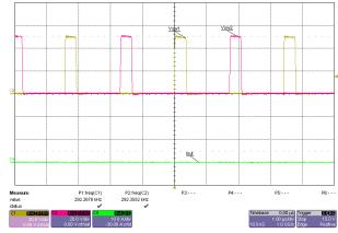
Figure 3-4. Switch Node Voltages, 48V Input, No Load, PFM Mode
