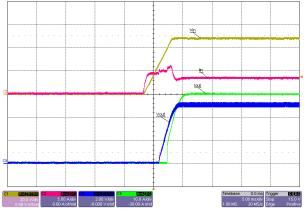
Figure 3-24. Start-Up Into No Load, 48V Input
