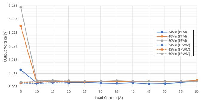
Figure 2-11. Load Regulation (5A to 60A Load)
