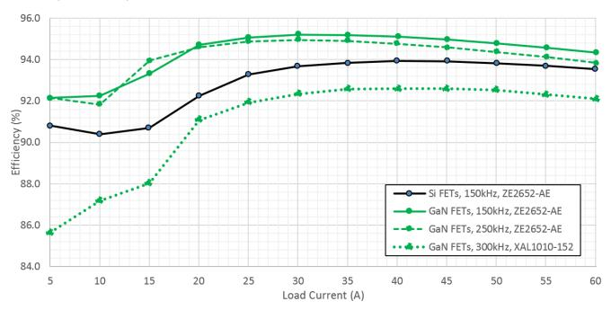
Figure 3-29. Efficiency Comparison Between Silicon and GaN FET Solutions at Varying Switching Frequencies (5A to 60A Load)
