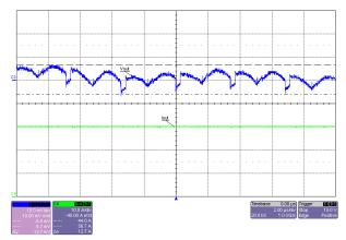
Figure 3-18. Output Voltage Ripple, 60V Input, 30A Load
