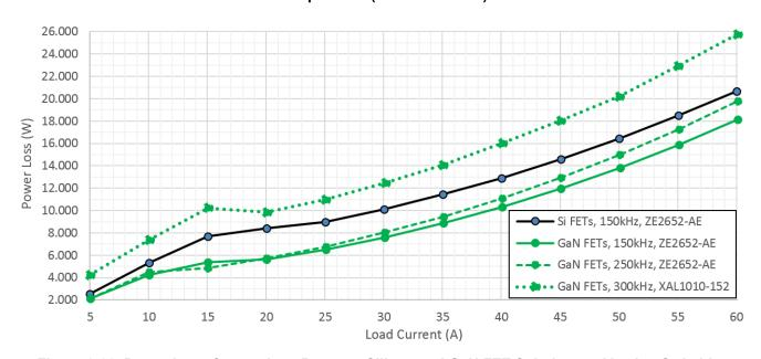
Figure 3-30. Power Loss Comparison Between Silicon and GaN FET Solutions at Varying Switching Frequencies (5A to 60A Load)
