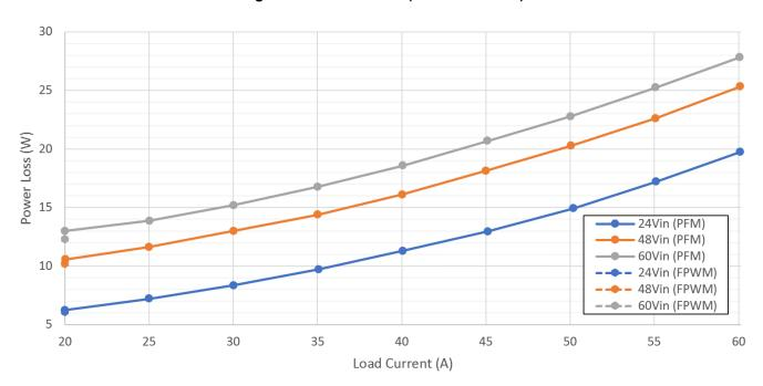
Figure 2-8. Power Loss (20A to 60A Load)
