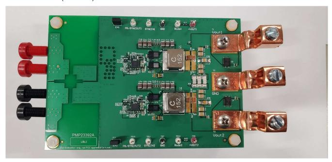
Figure 2-14. Top of PMP23392 Board
