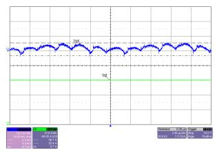
Figure 3-15. Output Voltage Ripple, 48V Input, 30A Load
