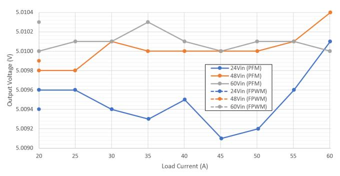
Figure 2-12. Load Regulation (20A to 60A Load)
