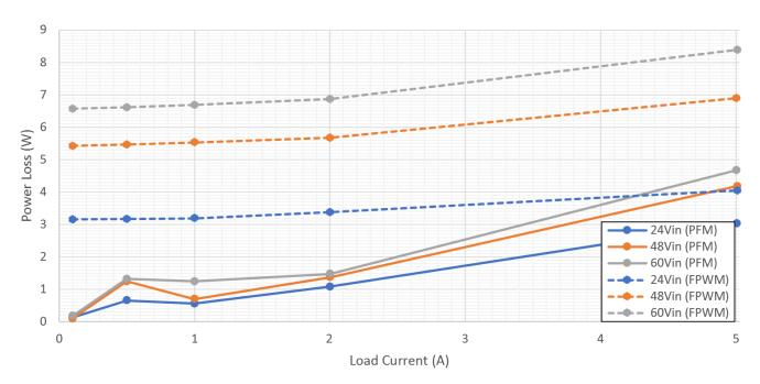
Figure 2-6. Power Loss (0A to 5A Load)
