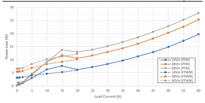
Figure 2-5. Power Loss (0A to 60A Load)
