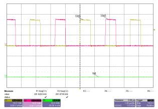
Figure 3-1. Switch Node Voltages, 24V Input, No Load, PFM Mode
