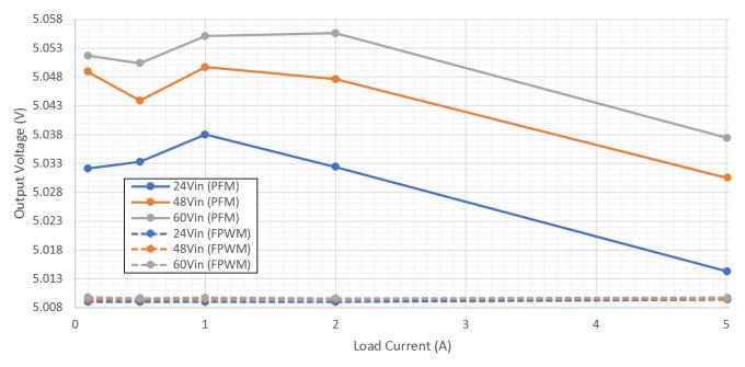
Figure 2-10. Load Regulation (0A to 5A Load)
