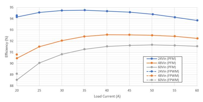
Figure 2-4. Efficiency (20A to 60A)
