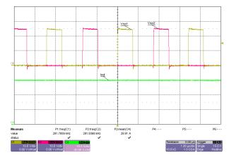
Figure 3-3. Switch Node Voltages, 24V Input, 30A Load
