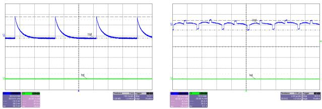
Figure 3-16. Output Voltage Ripple, 60V Input, No Load, PFM Mode
