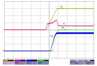
Figure 3-26. Start-Up Into No Load, 60V Input
