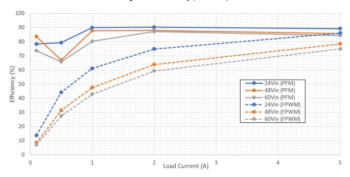
Figure 2-2. Efficiency (0A to 5A)
