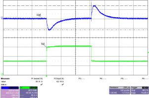
Figure 3-19. Load Transient Response, 24V Input, 30A-to-60A Load Step
