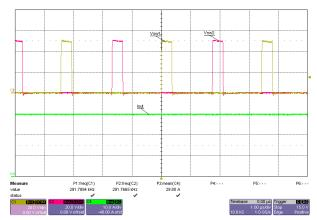
Figure 3-6. Switch Node Voltages, 48V Input, 30A Load
