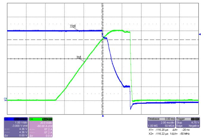
Figure 3-28. Overcurrent Protection at 48V Input
