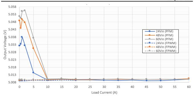
Figure 2-9. Load Regulation (0A to 60A Load)
