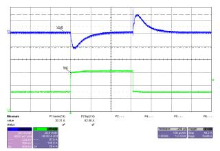
Figure 3-21. Load Transient Response, 60V Input, 30A-to-60A Load Step
