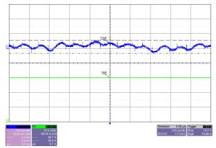
Figure 3-12. Output Voltage Ripple, 24V Input, 30A Load
