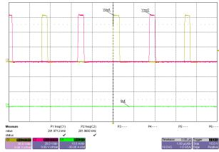
Figure 3-7. Switch Node Voltages, 60V Input, No Load, PFM Mode
