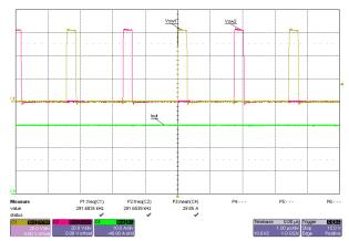
Figure 3-9. Switch Node Voltages, 60V Input, 30A Load
