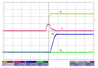
Figure 3-22. Start-Up Into No Load, 24V Input
