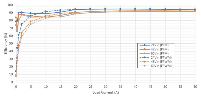
Figure 2-1. Efficiency (0A to 60A)
