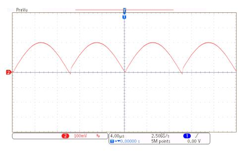
Figure 13: Measured output with 400 mVpp at 50 kHz sine-wave input
