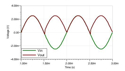
Figure 8: TINA-TITM simulated output at 1 kHz with 5mVpp sine-wave input
