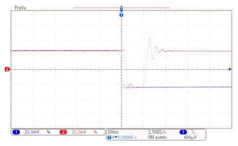
Figure 16: Measured output step response at input 50 mVpp and 1 kHz
