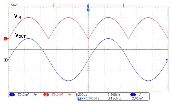
Figure 1: Measured output transient waveform with 1 kHz, 100 mVpp input signal
