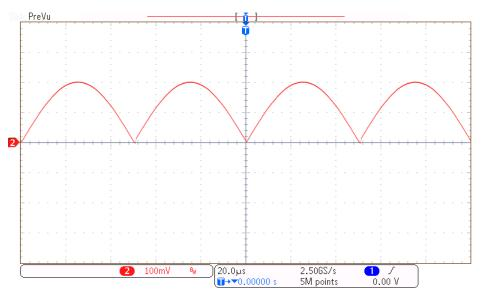
Figure 21: Measured output with 400 mVpp at 10 kHz sine-wave input
