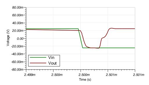
Figure 10: TINA-TI<sup>™</sup> simulated output step response at input of 50 mVpp
