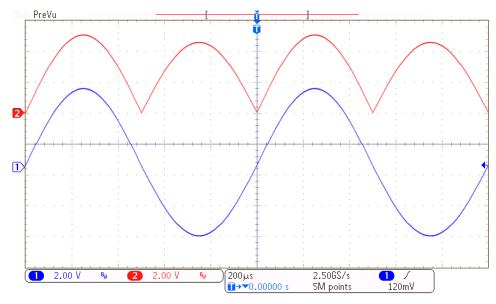
Figure 18: Output at 1 kHz with 4.95 Vp sine-wave input of the circuit without input buffer
