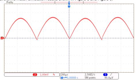
Figure 14: Measured output with 5 mVpp at 1 kHz sine-wave input
