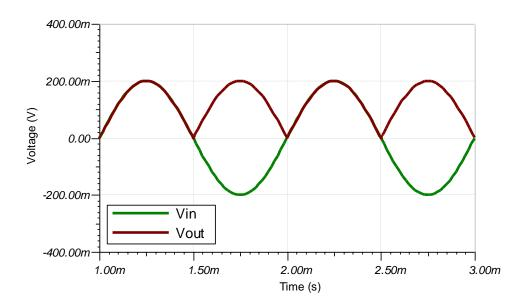
A. Transient simulation with +/- 200 mV at 1 kHz sinusoid wave input
