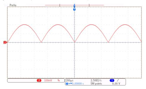
Figure 12: Measured output with 400 mVpp at 1 kHz sine-wave input
