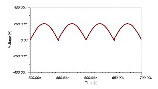
B. Simulated output with +/- 200 mV at 10 kHz sinusoid wave input Figure 20: TINA-TITM simulated transient waveform at 10 kHz with +/- 200 mV sine-wave input
