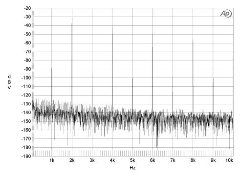
Figure 17: FFT of output at 1 kHz with 400 mVpp sine-wave input
