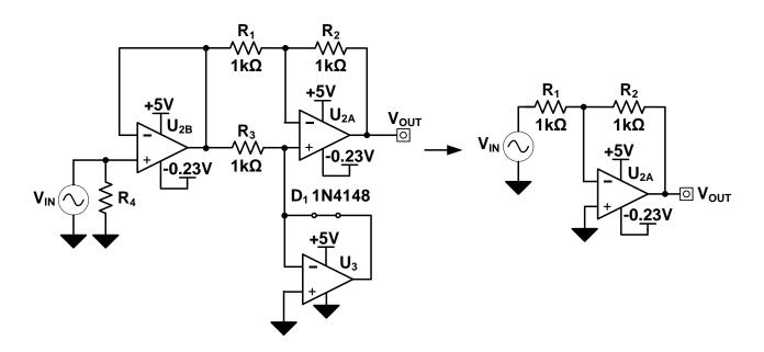
Figure 4: Simplified circuit with a negative input signal
