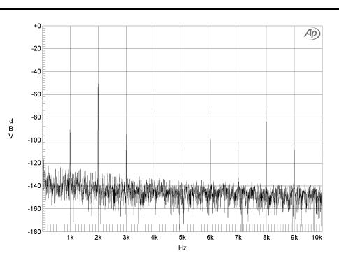
Figure 22: FFT of output at 1 kHz with 50 mVpp sine-wave input
