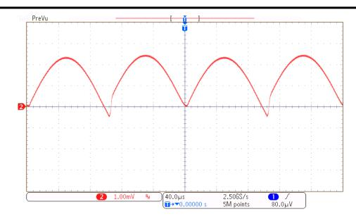
Figure 15: Measured output with 5 mVpp at 5 kHz sine-wave input
