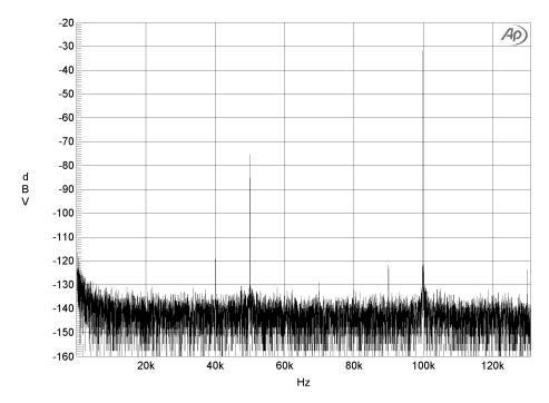
Figure 23: FFT of output at 50 kHz with 400 mVpp sine-wave input
