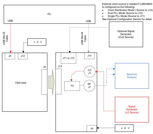
Figure 13. TSW1400 and TSW3085 Test Setup Block Diagram
