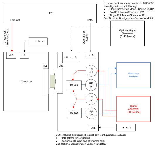
Figure 21. TSW3100 and TSW3084/TSW30H84 Test Setup Block Diagram
