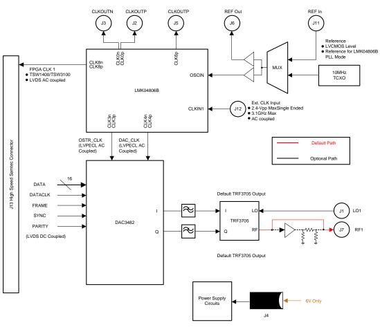
Figure 2. TSW3085EVM Block Diagram
