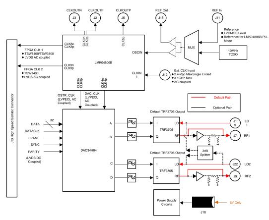
Figure 3. TSW30H84EVM Block Diagram
