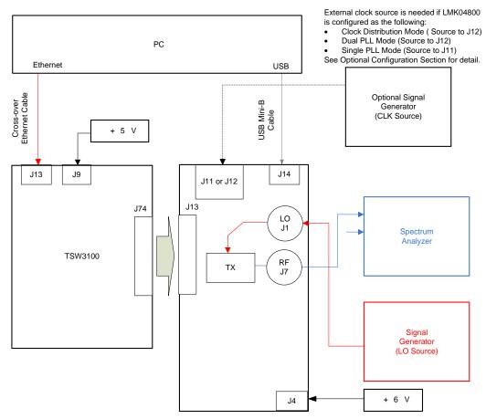
Figure 22. TSW3100 and TSW3085 Test Setup Block Diagram
