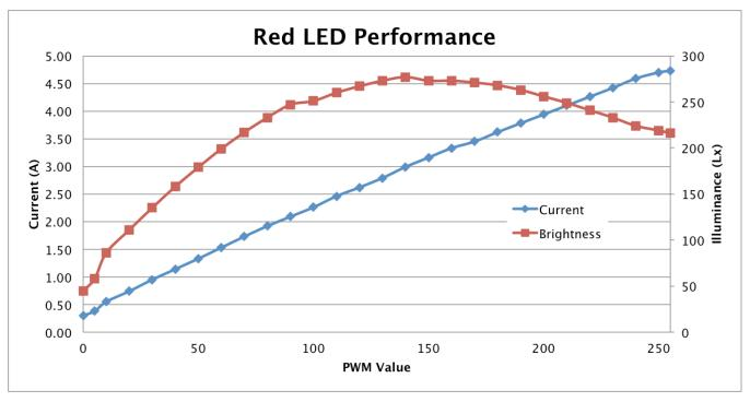
Figure 1-1. Typical Red LED Current and Illuminance based on PWM values
