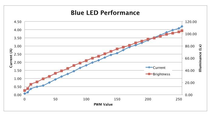
Figure 1-3. Typical Blue LED Current and Illuminance based on PWM values
