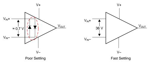
Figure 16. Selecting Amplifier for Fast Settling
