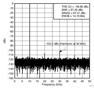
Figure 35. Measurement Result for FFT—Channel 0
