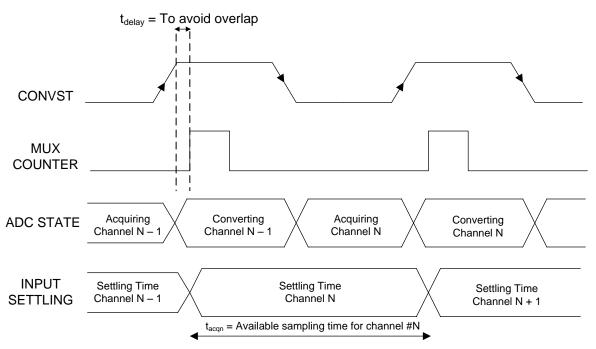
Figure 11. Multiplexed DAQ Timing Diagram
