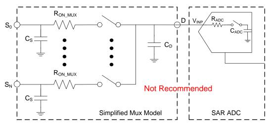
Figure 6. Low Output Impedance at MUX Output Introduces Distortion With SAR ADC (Not Recommended)
