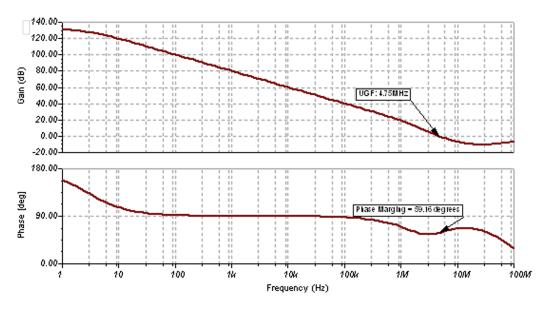
Figure 22. TINA-TI™ Schematic Result—AC Magnitude and Phase Plot for Input Drivers
