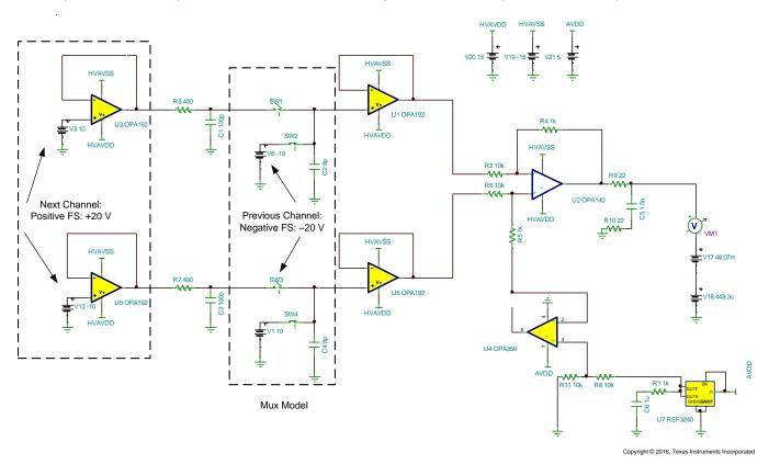
Figure 25. TINA-TI™ Schematic for Checking Settling Performance During Worst-Case Channel Switching
