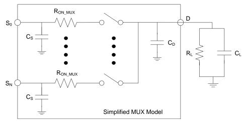
Figure 13. Simplified Model of a Multiplexer
