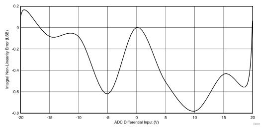
Figure 31. Measurement Result—ADC Integral Nonlinearity Error (INL) Plot (11 Points)
