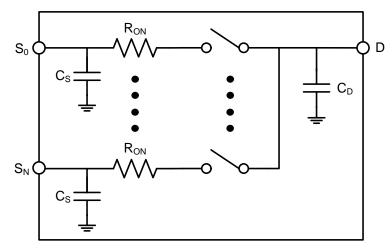
Figure 3. Simplified Multiplexer Model
