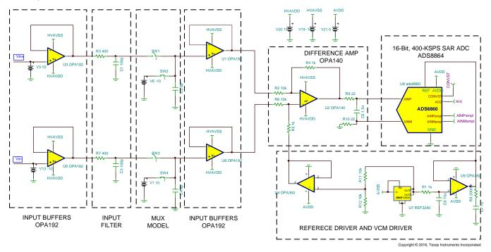
Figure 20. TINA-TI™—Schematic Showing Complete DAQ Block
