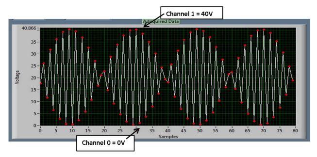
Figure 34. Measurement Result: Input Signal of 40 V<sub>pk-pk</sub> at 10 kHz—Alternating Channels Out of Phase
