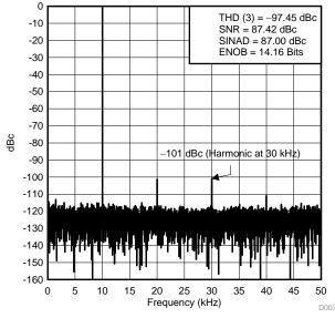
Figure 36. Measurement Result for FFT—Channel 1
