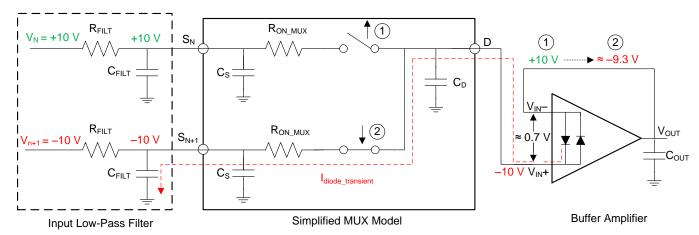
Figure 15. Back-to-Back Diode in Traditional Op Amp Introduces Settling Time Delay
