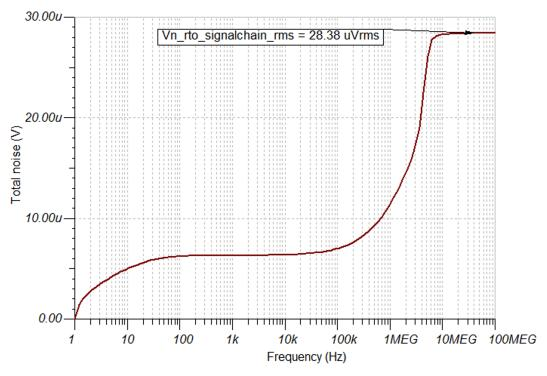
Figure 24. TINA-TI™ Schematic Result—Integrated AFE RMS Noise
