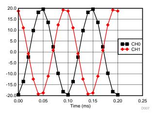
Figure 32. Input Signal of 40 V<sub>pk-pk</sub> at 10 kHz—Alternating Channel 0 and Channel 1 Out of Phase For Worst-Case Scenario
