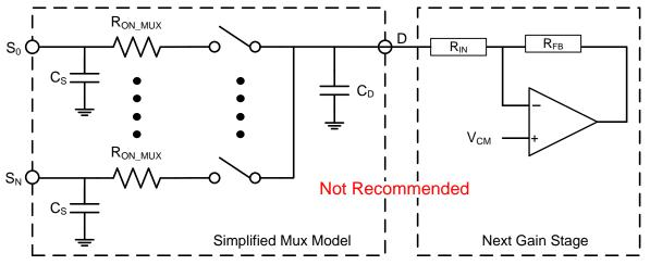
Figure 5. Low Output Impedance at MUX Output Introduces Distortion With Next Gain Stage (Not Recommended)
