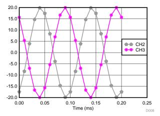
Figure 33. Input Signal of 40 V<sub>pk-pk</sub> at 10 kHz—Alternating Channel 2 and Channel 3 Out of Phase For Worst-Case Scenario
