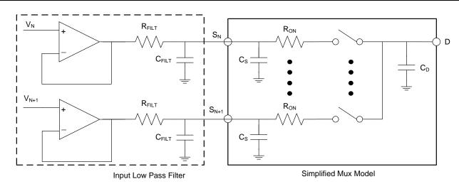
Figure 4. Charge Transfer Between Input Low-Pass Filter and Multiplexer Drain Capacitance
