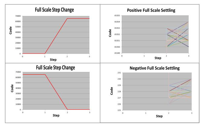
Figure 30. Measurement Result—Settling Time Performance for Full-Scale Step
