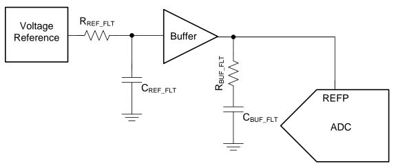
Figure 19. Simplified Schematic of Reference Driver Circuit
