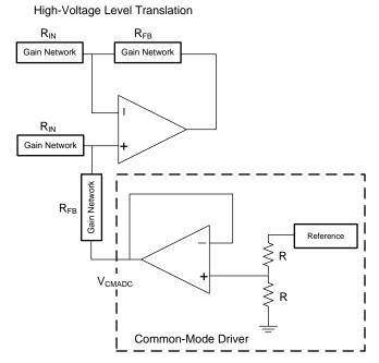
Figure 9. Difference Amplifier Common-Mode Driver
