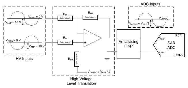
Figure 8. High-Voltage Level Translation Stage
