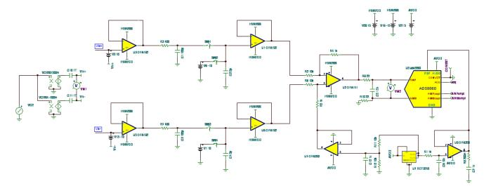
Figure 23. TINA-TI™—Schematic for Checking AFE Noise
