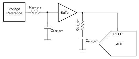
Figure 17. Simplified Schematic of Single-Ended Input Sampling Stage
