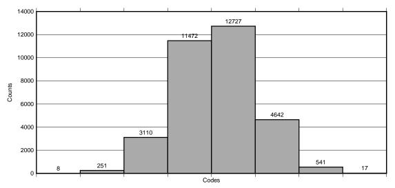
Figure 29. Measurement Result—Histogram Showing DC Noise (Mid-Scale)
