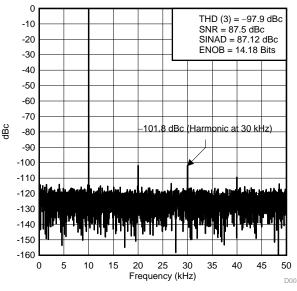
Figure 38. Measurement Result for FFT—Channel 3
