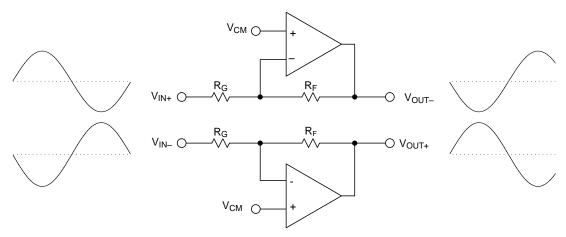
Figure 6. Differential-to-Differential Using a Dual Amplifier
