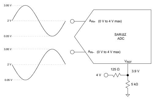
Figure 10. V<sub>REF</sub> Reduced to Avoid Saturation
