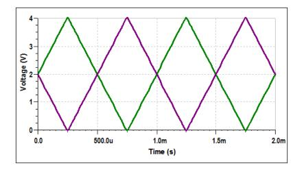
Figure 14. Unclipped Output with Negative Supply Connected to LM7705
