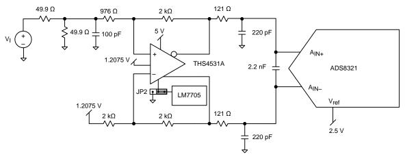
Figure 23. Driving ADS8321 With THS4531A
