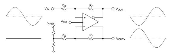
Figure 8. Single-Ended-to-Differential Using a Fully Differential Amplifier
