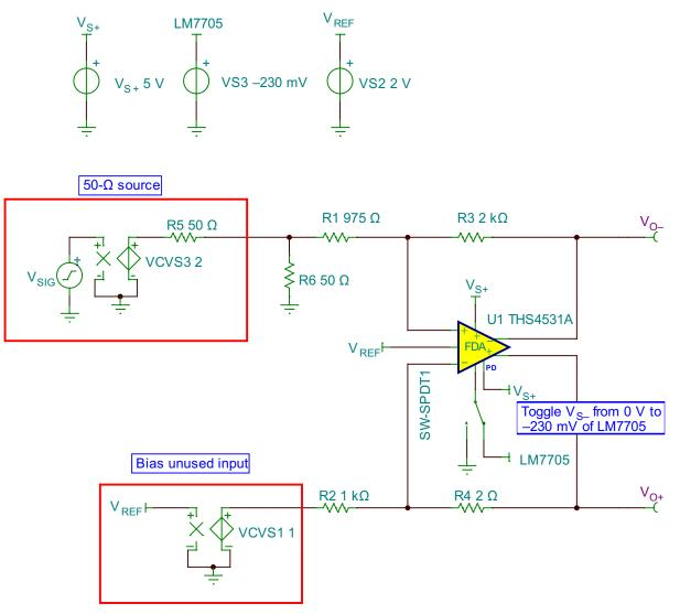
Figure 11. Schematic to Test the Impact of a Negative Supply
