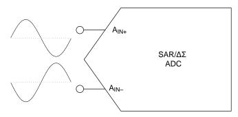
**Figure 5. Differential Input ADC**
