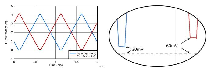
Figure 21. Measured Data with Negative Supply Connected to Ground
