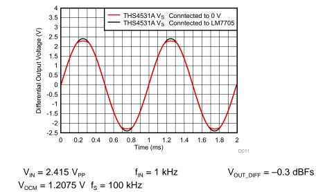
Figure 24. Time-Domain Capture of 1kHz Sine Wave using THS4531A and ADS8321 With and Without LM7705
