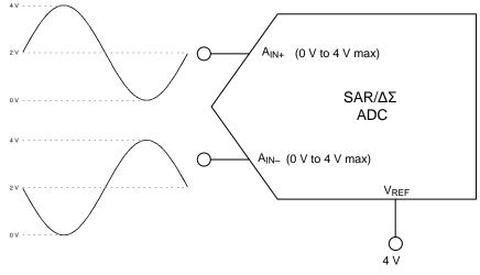
Figure 9. ADC Input Range Defined by V<sub>REF</sub>
