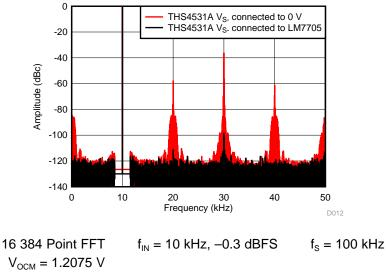
Figure 25. FFT of 10 kHz Sine Wave Using THS4531A and ADS8321 With and Without LM7705
