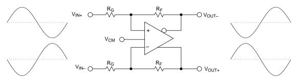
Figure 7. Differential-to-Differential Using a Fully Differential Amplifier
