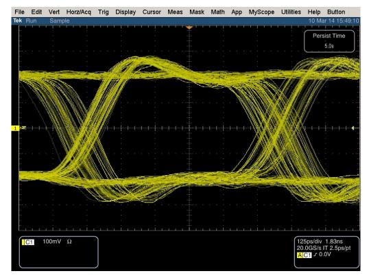
Figure 1: Eye diagram of DS90UB914A-CXEVM and DS90UB913A-CXEVM
