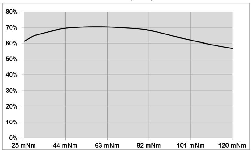
Power Efficiency vs Torque
