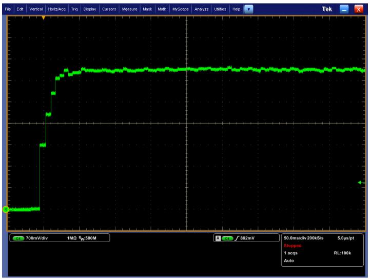
Motor speed was measured from the frequency of one Hall signal, and converted to this an analog waveform. Spin-up time was 60ms. The steady-state value represents 2054 RPM.
