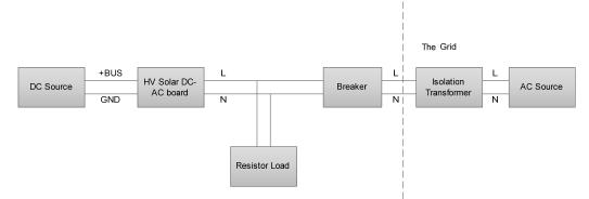
Fig 2.1 The connection of the test
