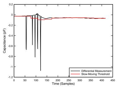
Figure 18. Response of Differential Measurement and Slow-Moving Threshold to Water Droplet Testing on Proximity Sensor
