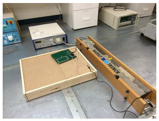
Figure 20. EFT Test Setup
