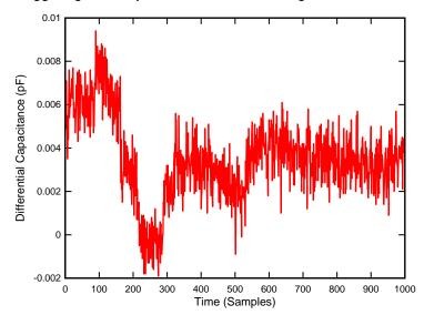
Figure 22. FDC1004 Output During High-Frequency Radiated Immunity Test
