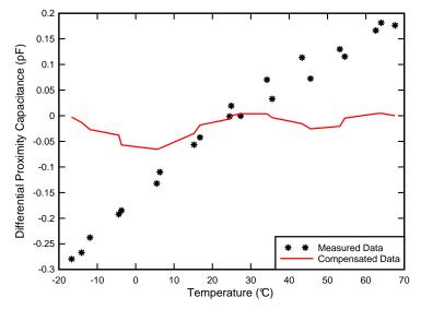
Figure 16. Corrected FDC1004 Baseline Capacitance versus Temperature
