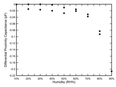
Figure 17. Baseline Capacitance versus Humidity
