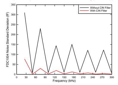
Figure 21. FDC1004 Noise versus Frequency of Radiated Interference
