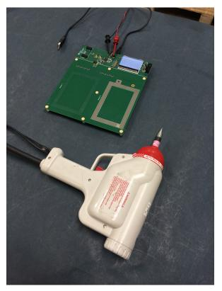
Figure 19. ESD Test Setup
