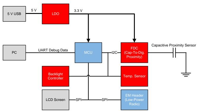
Figure 2. Capacitive-Based Human Proximity Detection System Block Diagram
