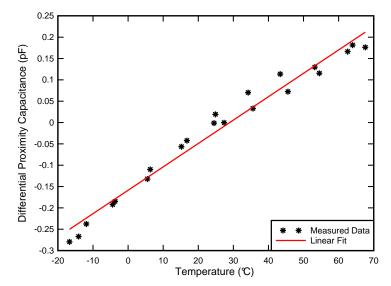
Figure 15. FDC1004 Baseline Capacitance versus Temperature
