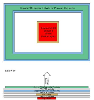
Figure 1. Capacitive Sensor Stackup
