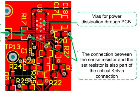
Figure 106. Layout Guideline for TPS24750 eFuse
