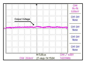
Figure 31. Output Voltage Ripple with 24 Vin, 10 Vout at 100-mA Load
