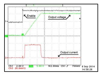
Figure 62. Inrush-Current Limitation with 24 Vin, 15 Vout, and 100- $\mu$ F Capacitive Load at 85°C
