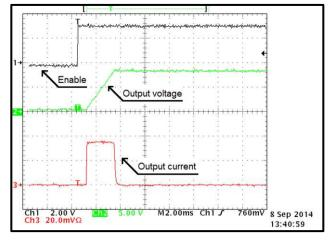
Figure 57. Inrush-Current Limitation with 24 Vin, 8 Vout, and 100-µF Capacitive Load at 25°C
