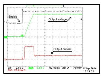
Figure 82. Start-Up at 24 Vin, 15 Vout with 150  $\Omega$  and 47- $\mu F$  Load at 85°C
