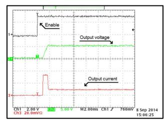
Figure 76. Start-Up at 24 Vin, 5 Vout with 51  $\Omega$  and 47-μF Load at 85°C
