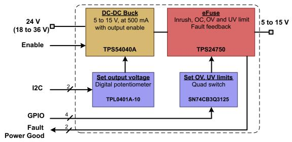
Figure 4. System Block Diagram of TIDA-00180
