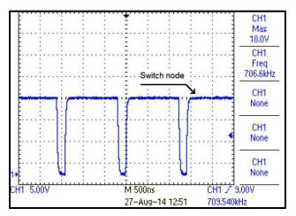
Figure 47. Switch Node Voltage with 18 Vin, 15 Vout at 300-mA Load
