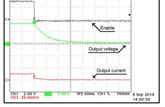
Figure 85. Shutdown at 24 Vin, 8 Vout with 82  $\Omega$  and 47- $\mu F$  Load at 25°C
