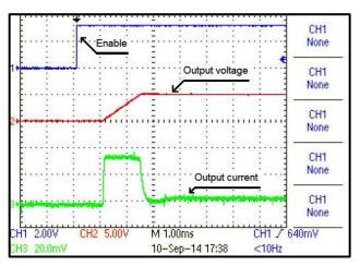
Figure 91. Output Voltage and Current Ramp-Up of TIDA-00180 Power Supply Configured to 5 V with GBPAS BiSS-C Encoder (Baumer)
