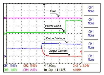
Figure 73. Fault and PG Signals during an OV Condition: 5 to 8 Vout at 100-mA Load
