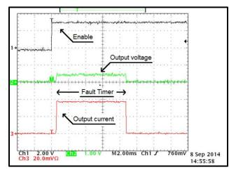
Figure 54. eFuse OC Protection with Disconnect after 8 ms with 24 Vin, 15 Vout and 1-Ω load at 85°C
