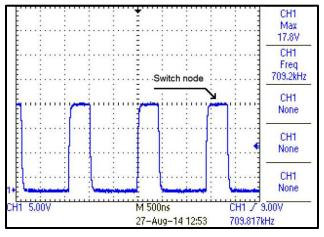
Figure 35. Switch Node Voltage with 18 Vin, 5 Vout at 300-mA Load
