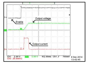
Figure 55. Inrush-Current Limitation with 24 Vin, 5 Vout, and 100-µF Capacitive Load at 25°C
