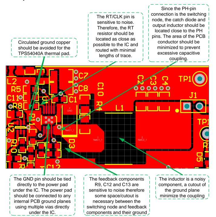
Figure 105. Layout Guidelines for TPS54040A
