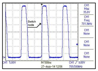
Figure 44. Switch Node Voltage with 36 Vin, 10 Vout at 30-mA Load
