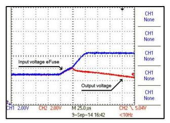
Figure 63. 6-V OV Event at 25°C, Voltage Step from 5 to 8 V at 100 mA
