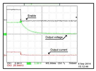
Figure 86. Shutdown at 24 Vin, 8 Vout with 82  $\Omega$  and 47-µF Load at 85°C
