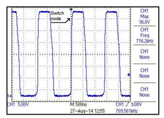
Figure 48. Switch Node Voltage with 36 Vin, 15 Vout at 30-mA Load
