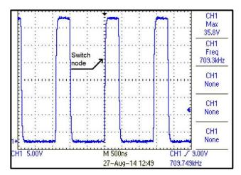
Figure 42. Switch Node Voltage with 36 Vin, 10 Vout at 300-mA Load
