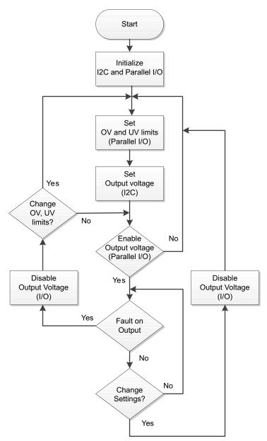
Figure 17. Flowchart for Voltage and Protection Limits Configuration
