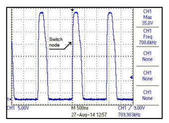
Figure 40. Switch Node Voltage with 36 Vin, 8 Vout at 30-mA Load
