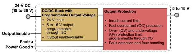
Figure 2. Block Diagram of the Power Supply with Programmable Output Voltage and Protection
