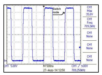
Figure 46. Switch Node Voltage with 36 Vin, 15 Vout at 300-mA Load
