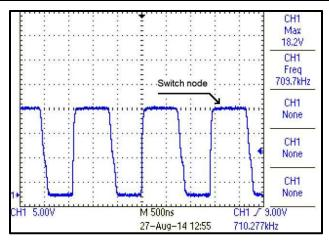
Figure 45. Switch Node Voltage with 18 Vin, 10 Vout at 30-mA Load
