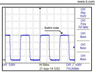
Figure 39. Switch Node Voltage with 18 Vin, 8 Vout at 300-mA Load
