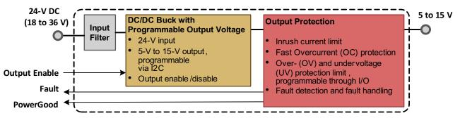
Figure 5. Block Diagram of Power Supply with Programmable Output Voltage and Protection
