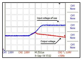
Figure 64. 6-V OV Event at 85°C, Voltage Step from 5 to 8 V at 100-mA Load
