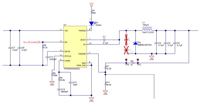
Figure 7. Schematic of DC-DC Buck Converter with TPS54040A
