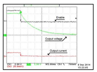
Figure 90. Shutdown at 24 Vin, 15 Vout with 150  $\Omega$  and 47- $\mu F$  Load at 85°C
