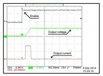
Figure 56. Inrush-Current Limitation with 24 Vin, 5 Vout, and 100-µF Capacitive Load at 85°C
