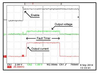
Figure 51. eFuse OC Protection with Disconnect after 10 ms with 24 Vin, 5 Vout and 1- $\Omega$  load at 25°C
