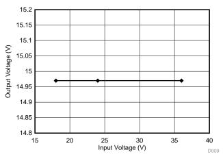
Figure 28. Output Voltage versus Input Voltage at 15 Vout and 66-mA load
