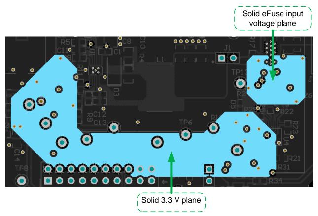
Figure 108. Supply Voltage Layer
