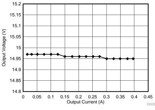
Figure 24. Output Voltage versus Output Current at 24 Vin and 15 Vout
