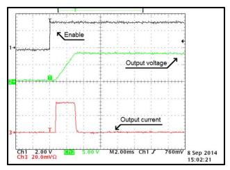
Figure 58. Inrush-Current Limitation with 24 Vin, 8 Vout, and 100-µF Capacitive Load at 85°C
