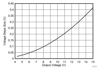
Figure 20. Voltage Steps Size versus Output Voltage
