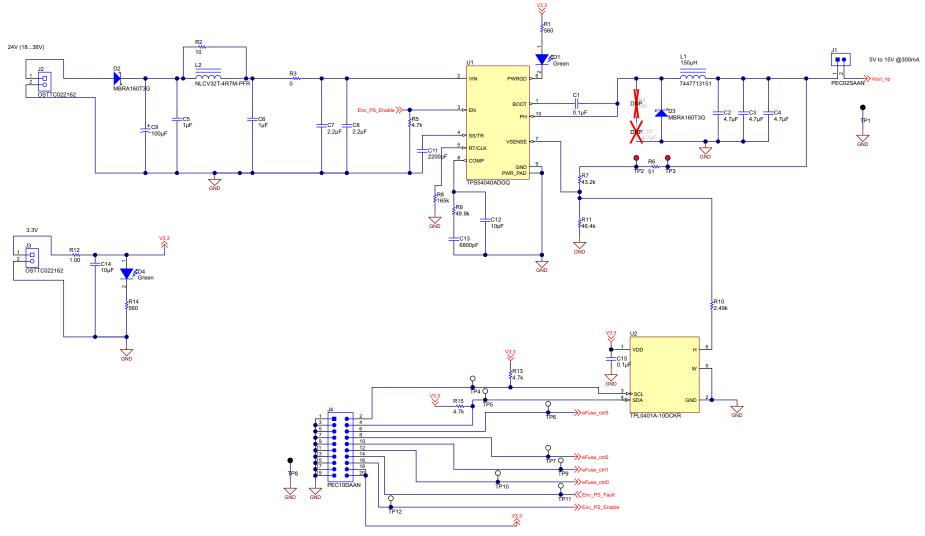
Figure 94. DC-DC Buck Converter with Programmable Output Voltage
