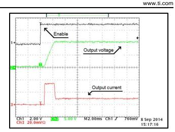
Figure 80. Start-Up at 24 Vin, 10 Vout with 100  $\Omega$  and 47- $\mu F$  Load at 85°C
