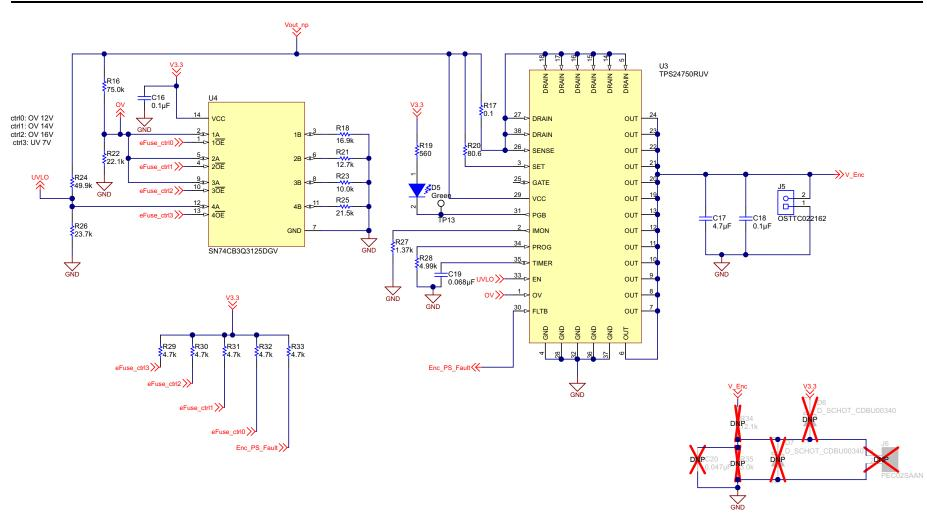
Figure 95. Output Protection with eFuse
