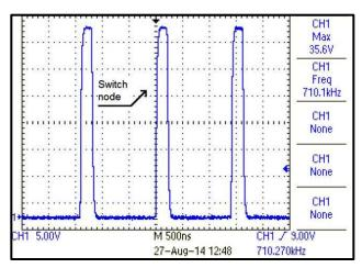
Figure 34. Switch Node Voltage with 36 Vin, 5 Vout at 300-mA Load
