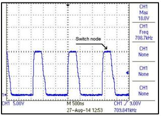
Figure 37. Switch Node Voltage with 18 Vin, 5 Vout at 30-mA Load
