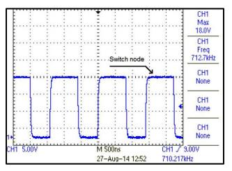
Figure 43. Switch Node Voltage with 18 Vin, 10 Vout at 300-mA Load
