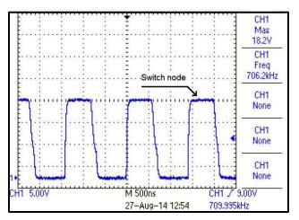
Figure 41. Switch Node Voltage with 18 Vin, 8 Vout at 30-mA Load
