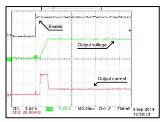
Figure 77. Start-Up at 24 Vin, 8 Vout with 82  $\Omega$  and 47-µF Load at 25°C
