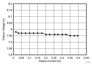
Figure 22. Output Voltage versus Output Current at 24 Vin and 8 Vout
