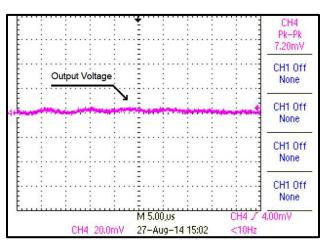
Figure 32. Output Voltage Ripple with 24 Vin, 15 Vout at 66-mA Load
