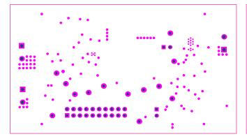
Figure 102. Bottom Solder Mask
