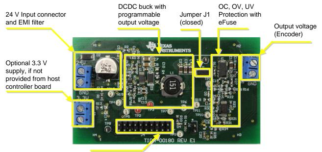
I/O connector (3.3 V I/O) for P/S configuration by host processor
