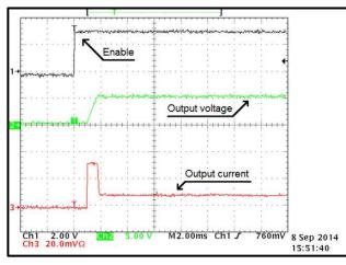
Figure 75. Start-Up at 24 Vin, 5 Vout with 51  $\Omega$  and 47-µF Load at 25°C
