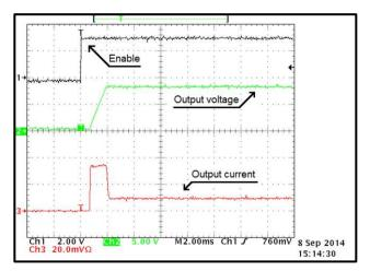
Figure 78. Start-Up at 24 Vin, 8 Vout with 82 Ω and 47-µF Load at 85°C
