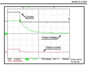
Figure 88. Shutdown at 24 Vin, 10 Vout with 100  $\Omega$  and 47-µF Load at 85°C
