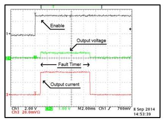
Figure 52. eFuse OC Protection with Disconnect after 8 ms with 24 Vin, 5 Vout and 1- $\Omega$  load at 85°C
