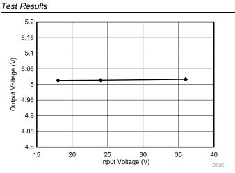
Figure 25. Output Voltage versus Input Voltage at 5 Vout and 200-mA load
