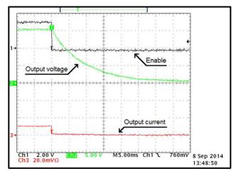
Figure 89. Shutdown at 24 Vin, 15 Vout with 150  $\Omega$  and 47- $\mu F$  Load at 25°C
