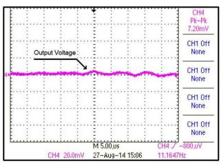
Figure 29. Output Voltage Ripple with 24 Vin, 5 Vout at 200-mA Load
