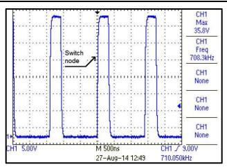
Figure 38. Switch Node Voltage with 36 Vin, 8 Vout at 300-mA Load
