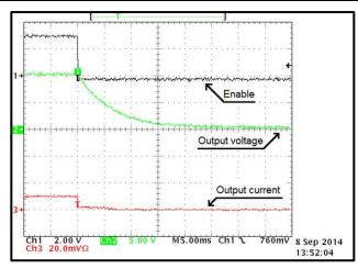
Figure 87. Shutdown at 24 Vin, 10 Vout with 100  $\Omega$  and 47- $\mu F$  Load at 25°C
