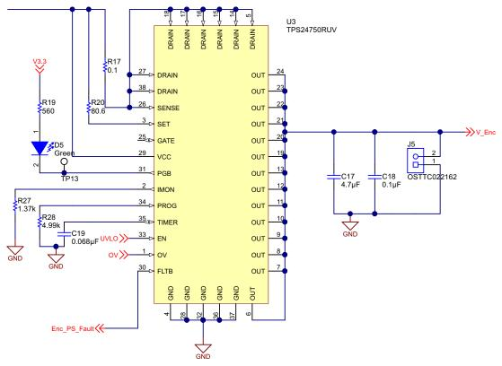
Figure 13. TPS24750 eFuse Schematic
