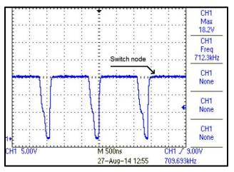
Figure 49. Switch Node Voltage with 18 Vin, 15 Vout at 30-mA Load
