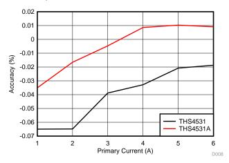
Figure 42. DC Accuracy Using THS4531 and THS4531A
