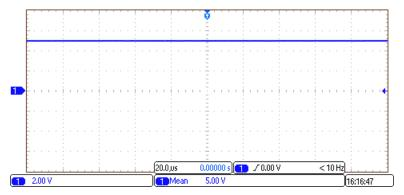
Figure 43. 5-V Signal from TPS7A4700
