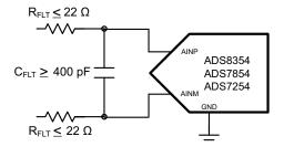
Figure 8. Anti-Aliasing Filter for ADS7x54
