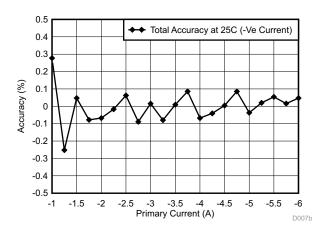
Figure 40. Total Accuracy Graph while Using Internal ADC of Delfino Controller for Positive Current (Left) for Negative Current (Right)
