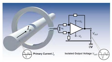
Figure 3. Open-Loop Fluxgate Sensor
