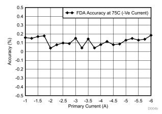
Figure 34. FDA Accuracy at 75°C for Positive Current (Left) for Negative Current (Right)
