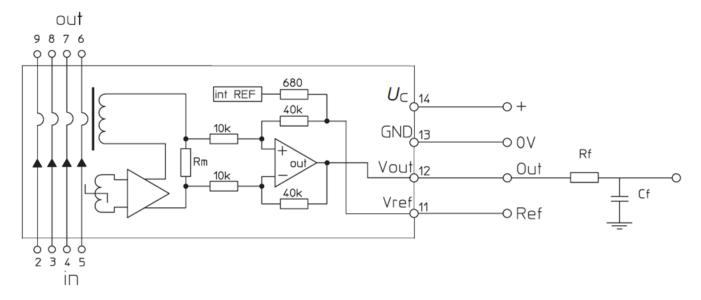
Figure 5. Internal Structure of CKSR 6-NP
