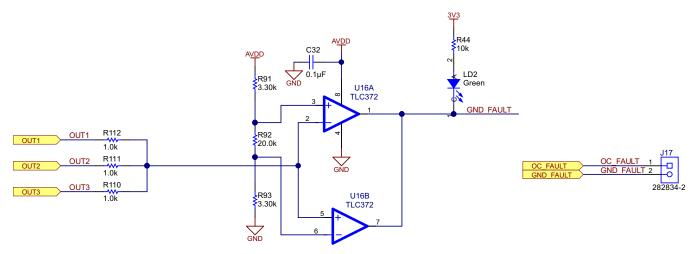
Figure 20. Earth Fault Protection Using TLC372
