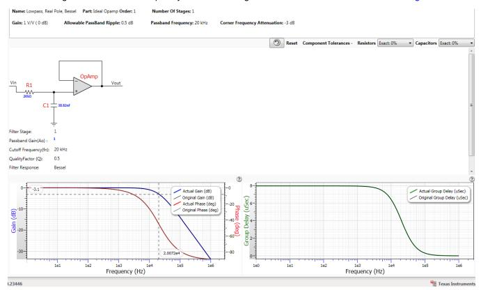
Figure 12. Low-Pass Filter Design Simulation Using FilterPro
