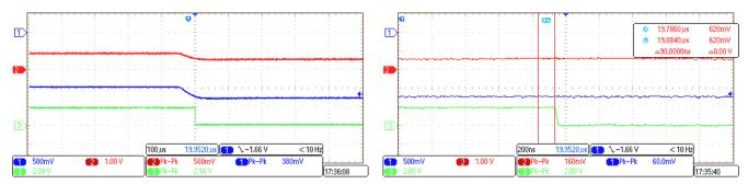
Figure 54. Earth Fault Detection at VTH (neg)
