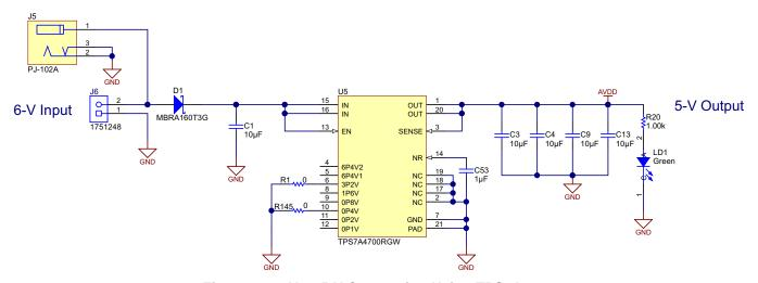
Figure 17. 6-V to 5-V Conversion Using TPS7A4700
