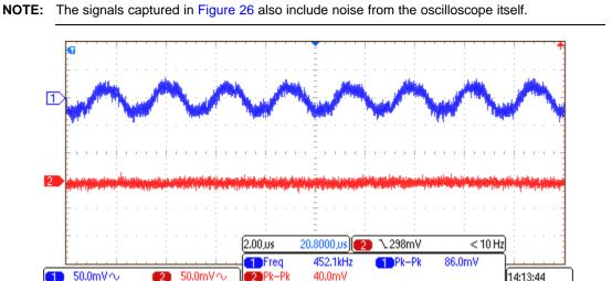
Figure 26. Noise Signal Before and After the Low-Pass Filter
