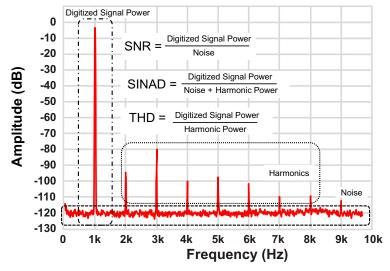
Figure 29. Typical FFT Plot Showing Different Dynamic Parameters
