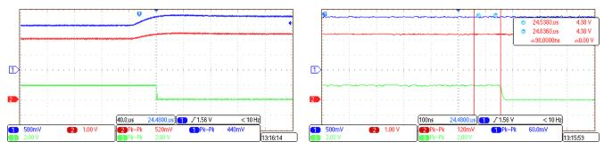
Figure 48. Overcurrent Detection at VTH (pos)
