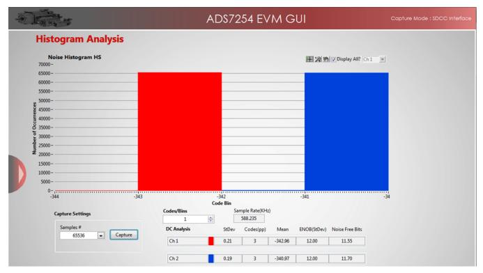
Figure 27. Histogram of Captures for Two Channels Using ADS7254 EVM GUI
