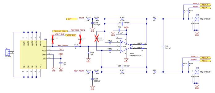
Figure 11. THS4531 FDA Interface Between Sensor and ADC
