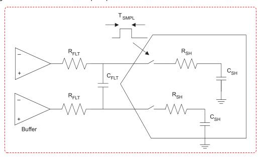
Figure 9. Input Capacitor C<sub>FLT</sub> for Attenuating Noise
