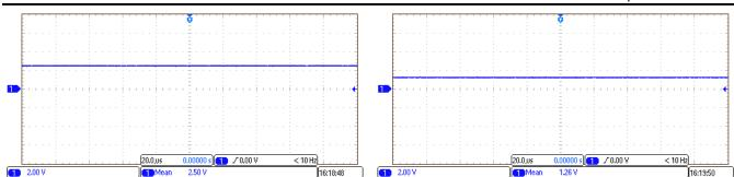
Figure 46. 2.5-V Reference Signal Generated by REF2025
