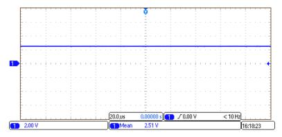
Figure 45. 2.5-V Reference Signal Generated by REF5025
