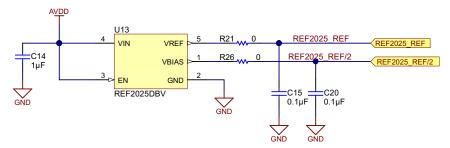
Figure 16. REF2025 Circuit to Provide 1.25 V and 2.5 V as Reference
