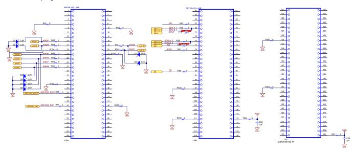
Figure 25. Schematic Capture for J15 and J16 (to Connect to 180-Pin Connector on Control Card)
