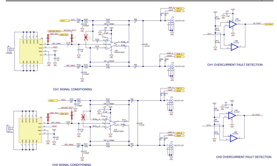
Figure 57. Channel 1 and 2 Schematic
