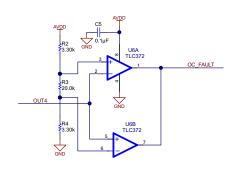
CH4 OVERCURRENT FAULT DETECTION
