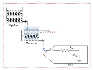
Figure 10. Filter Capacitor Delivering Charges to C<sub>SH</sub>
