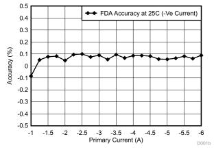
Figure 33. FDA Accuracy at 25°C for Positive Current (Left) for Negative Current (Right)
