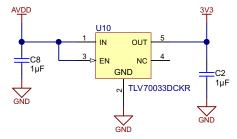
Figure 18. 5-V to 3.3-V Conversion Using TLV70033
