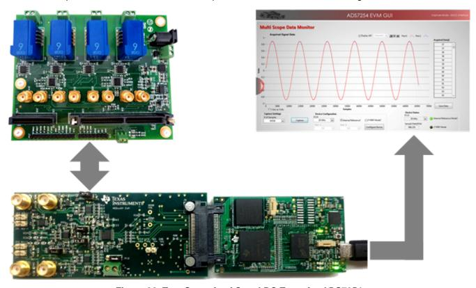
Figure 32. Test Setup for AC and DC Tests for ADS7254
