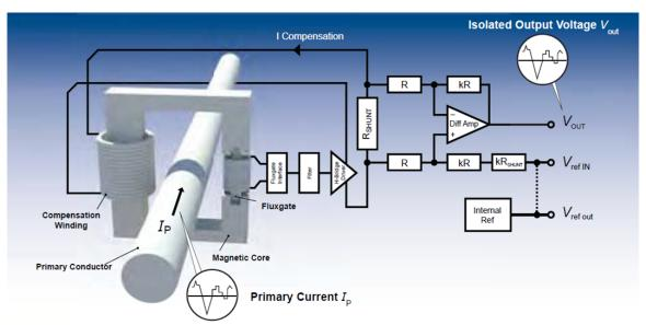
Figure 4. Close-Loop Fluxgate Sensor
