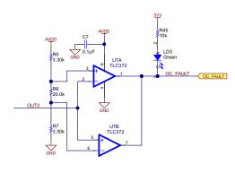
CH3 OVERCURRENT FAULT DETECTION
