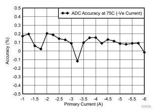
Figure 36. ADC Accuracy at 75°C for Positive Current (Left) for Negative Current (Right)
