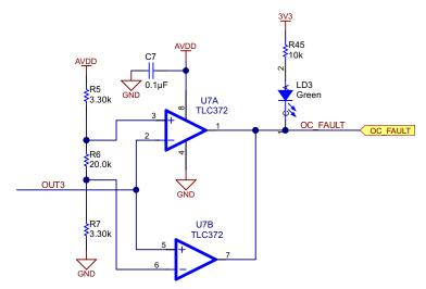
Figure 19. Overcurrent Protection Using TLC372
