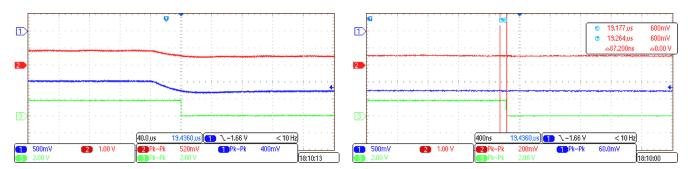
Figure 50. Overcurrent Detection at VTH (neg)
