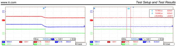
Figure 51. Earth Fault Detection at VTH (neg)
