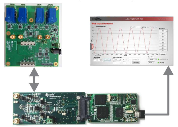
Figure 30. Test Setup for AC and DC Tests for ADS7253
