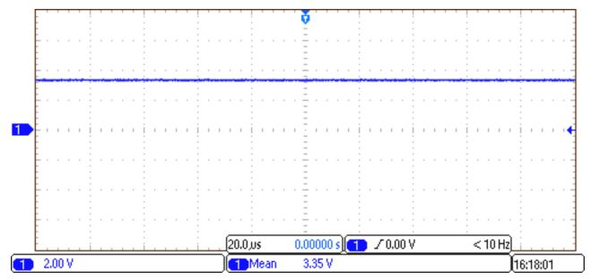
Figure 41. 3.3-V Reference Signal Generated by TLV70033
