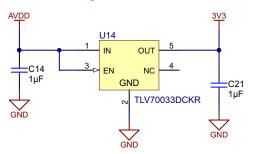
Figure 17. 5- to 3.3-V Conversion Using TLV70033
