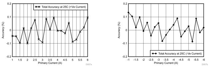
Figure 38. Total Accuracy While Using Internal ADC of Piccolo 28027 Controller (Left) for Positive Current (Right) for Negative Current
