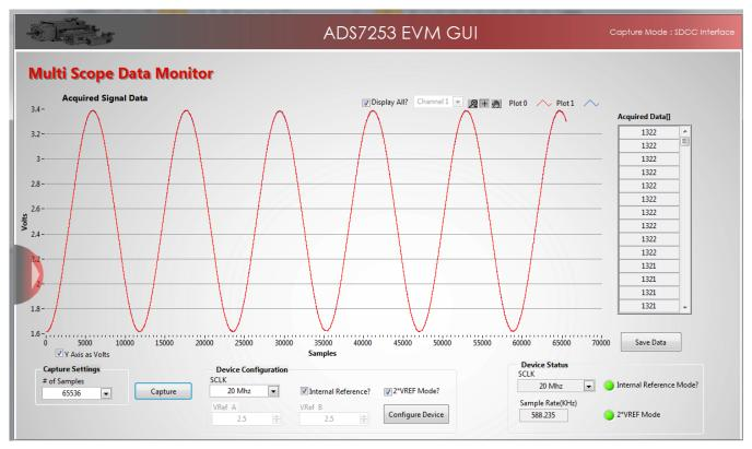
Figure 28. AC Signal Capture for Two Channels Using ADS7253 EVM GUI
