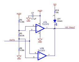
Figure 18. Overcurrent Protection Using TLC372
