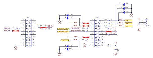
Figure 23. Schematic Capture for J11 and J14 (To Be Connected to 40-Pin Connector on LaunchPad)
