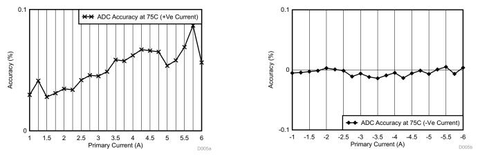
Figure 34. ADC Accuracy at 75°C (Left) for Positive Current (Right) for Negative Current
