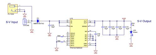
Figure 16. 6- to 5-V Conversion Using TPS7A4700
