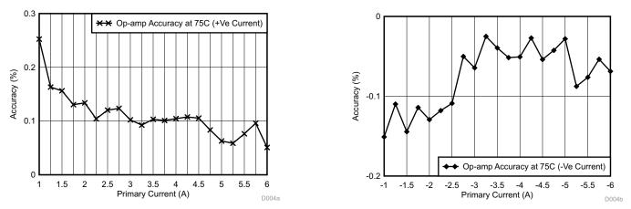
Figure 32. Op-Amp Accuracy at 75°C (Left) for Positive Current (Right) for Negative Current
