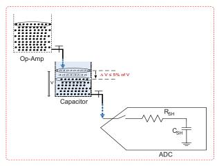
Figure 9. Filter Capacitor Delivering Charges to C<sub>SH</sub>
