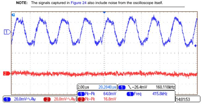
Figure 24. Noise Signal Before and After the Low-Pass Filter
