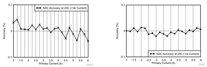
Figure 33. ADC Accuracy at 25°C (Left) for Positive Current (Right) for Negative Current
