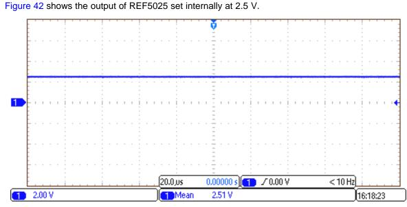
Figure 42. 2.5-V Reference Signal Generated by REF5025
