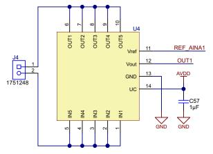
Figure 6. CKSR 6-NP with Capacitor Decoupling on Supply Pin
