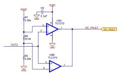
CH2 OVERCURRENT FAULT DETECTION
