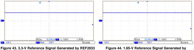
Figure 44. 1.65-V Reference Signal Generated by **REF2033**
