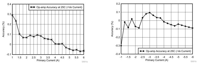
Figure 31. Op-Amp Accuracy at 25°C (Left) for Positive Current (Right) for Negative Current
