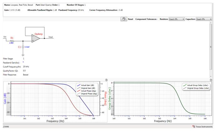
Figure 11. Low-Pass Filter Design Simulation Using FilterPro
