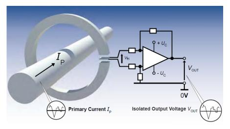
Figure 3. Open-Loop Fluxgate Sensor
