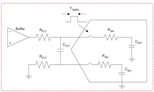
Figure 8. Input Capacitor C<sub>FLT</sub> for Attenuating Noise
