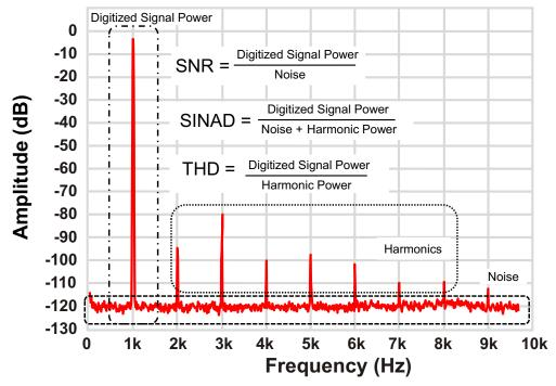
Figure 27. Typical FFT Plot Showing Different Dynamic Parameters
