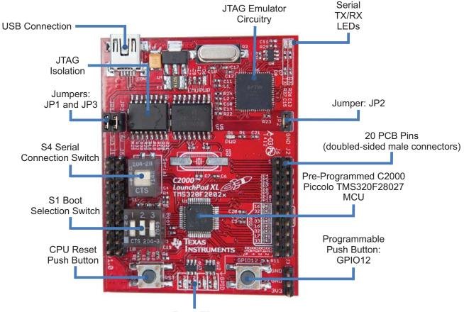
Four LEDs Figure 22. Image of LAUNCHXL-F28027
