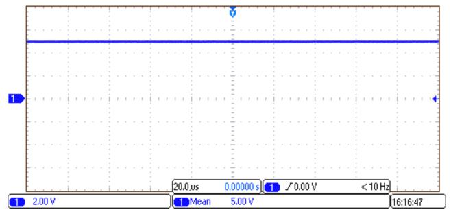
Figure 40. 5-V Signal From TPS7A4700
