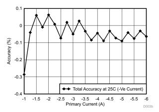
Figure 35. Total Accuracy at 25°C (Left) for Positive Current (Right) for Negative Current
