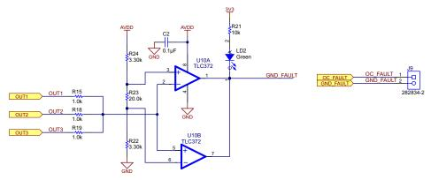
Figure 19. Earth Fault Protection Using TLC372
