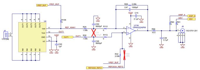
Figure 10. OPA4322 Interface Between Sensor and ADC
