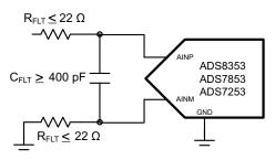
Figure 7. Anti-Aliasing Filter for ADS7x53
