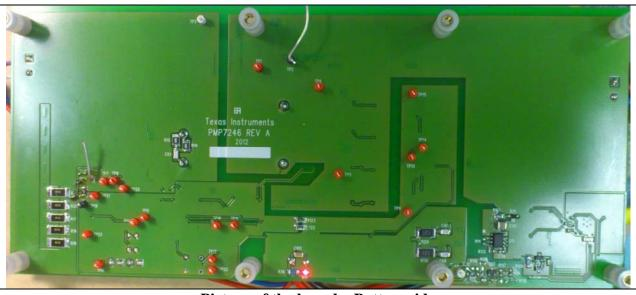
**Picture of the board – Bottom side** Dimensions: 217mm × 96mm
