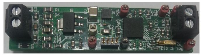
Figure 15. Top-Side PCB Assembly View
