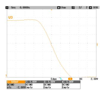
Hall sensor pulldown (open-drain output)
