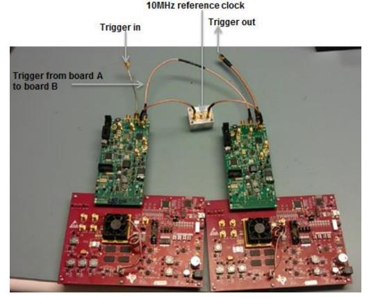
Figure 5: Setup of ADC12J4000 EVM and TSW14J56 EVM
