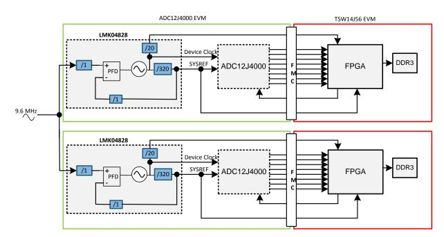
Figure 3: Block diagram of synchronized 2x ADC12J4000 and 2x TSW14J56
