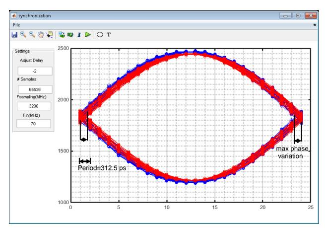
Figure 9: Eye diagram output of synchronized ADC12J4000 showing 1434 cycles of 70 MHz sinusoid
