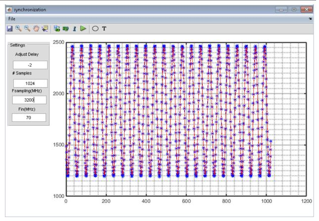
Figure 6: Main user Interface to control ADC12J4000 and TSW14J56 synchronization
