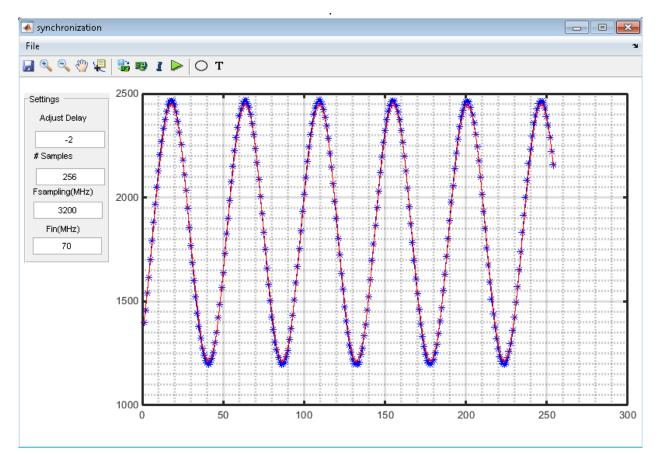
Figure 8: Time-Domain output of synchronized ADC12J4000 showing six cycles of 70 MHz sinusoid
