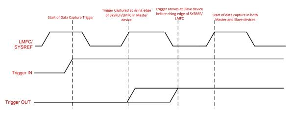
Figure 4: Trigger generation timing diagram
