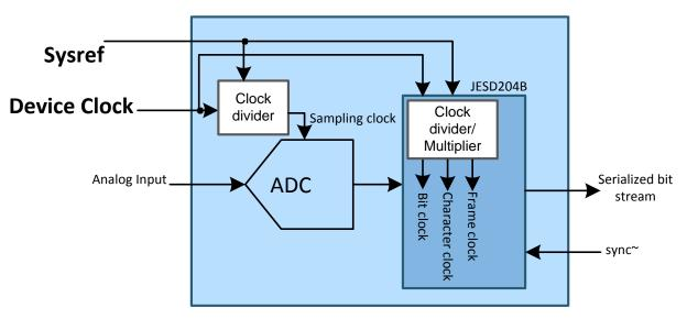
Figure 2: Clock generation in a JESD204B device
