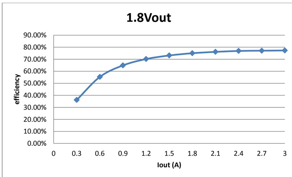
Figure 7. VIN = 12V, VCCAUX Efficiency
