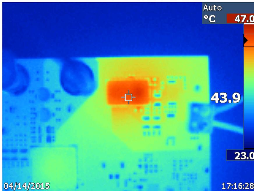
Figure 15. VIN = 12V, VCCAUX Thermal Image @ 3A
