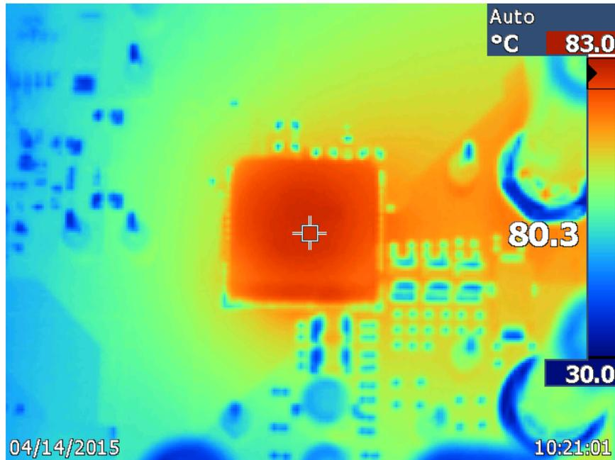
Figure 14. VIN = 12V, VCCINT Thermal Image @ 20A
