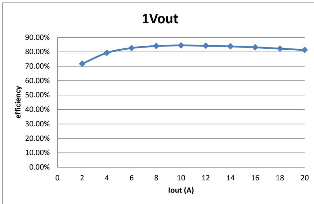
Figure 6. VIN = 12V, VCCINT Efficiency
