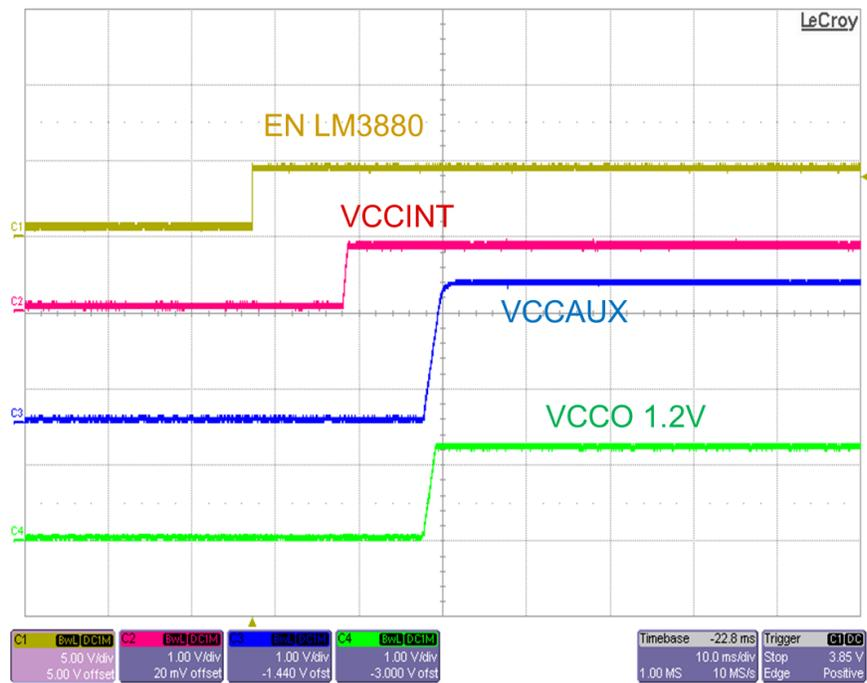
Figure 4. Startup Waveform
