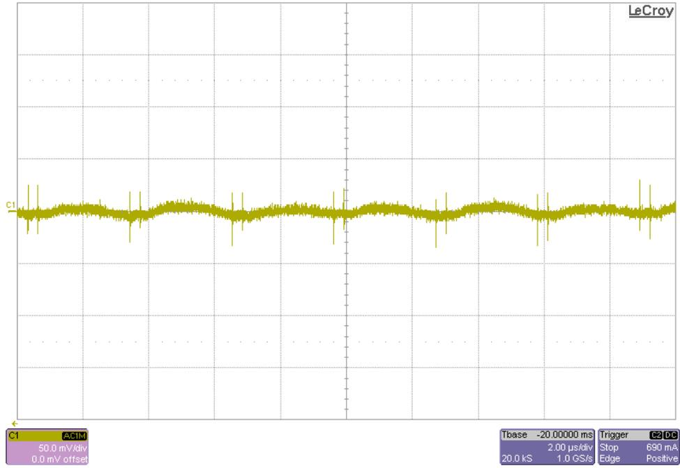
Figure 10. VIN = 12V, VCCINT Output Ripple @ IOOUT = 20A
