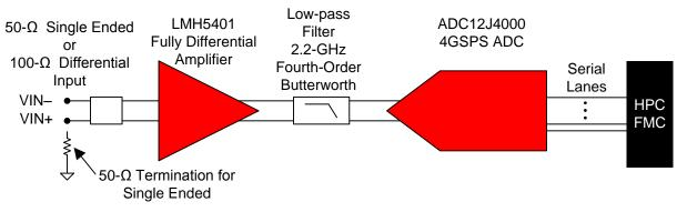
Figure 2. TSW12J54EVM Signal Path
