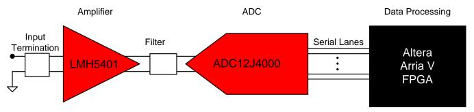
Figure 1. Simplified Block Diagram of RF Sampling ADC With DC-Coupled Front End
