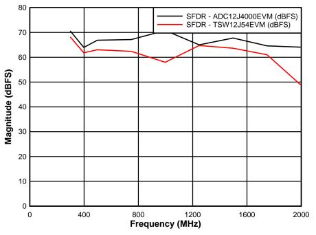
Figure 7. Comparison Between TSW12J54EVM and ADC12J4000EVM
