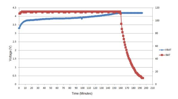
Plot shows 110mA constant current charge cycle powered by wireless power receiver.
