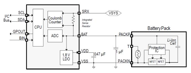
Battery detail specifications are necessary for better performance of gauging, or, characterize battery by Texas Instruments Gauge Development Kit (GDK) which is a complete evaluation system for any single-cell fuel.
